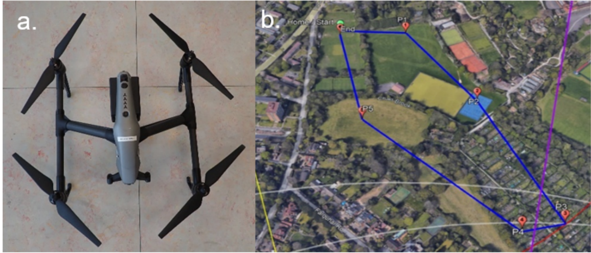
Figure 7.4: (a) DJI Inspire 3, target type used for controlled drone flights. (b) Flight path used for the experiments (Google maps).
