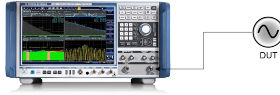
Figure B.1: Diagram of the setup for PN measurements. DUT - Device under test.
