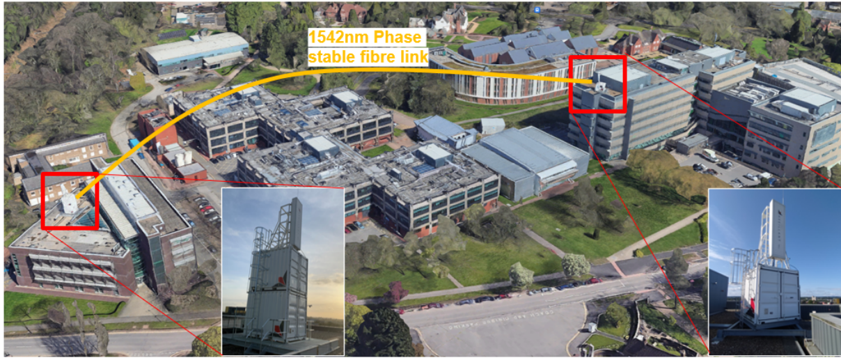
Figure 7.20: Overview of the L-band staring radar network setup for MWPO measurements and the phase noise stabilized fibre link (Google maps).
