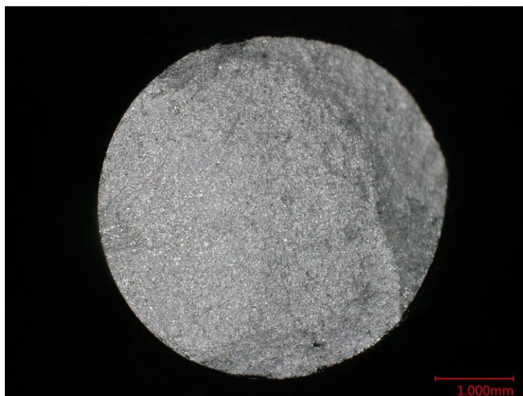
Figure D.14 Optical macrograph of the fracture surface of specimen HF010.
