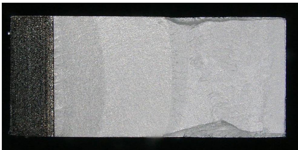
Figure D.44 Optical macrograph of the fracture surface of specimen CP015R.
