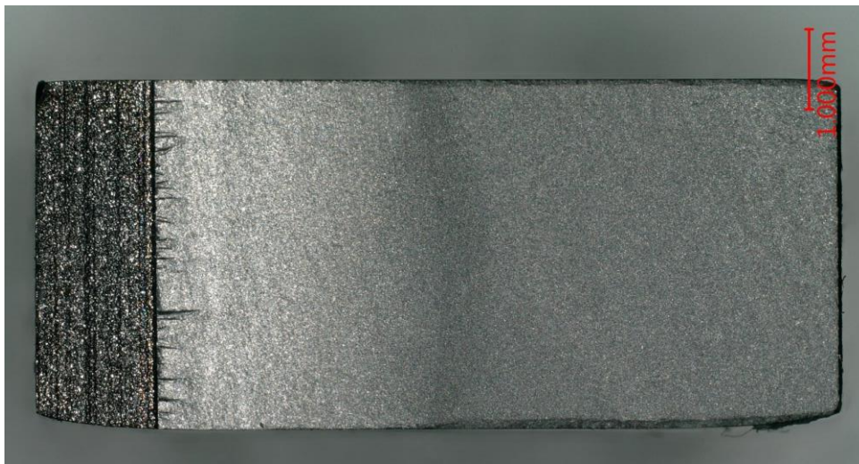
Figure D.41 Optical macrograph of the fracture surface of specimen CP013L.
