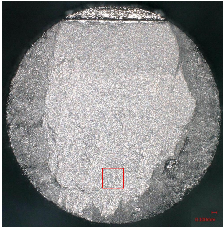
Figure E.13 Optical macrograph of the break-open fracture surface of HF022. The location of discovered HAPs is marked in the red box.
