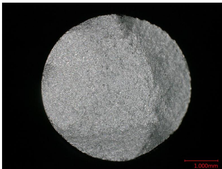
Figure D.17 Optical macrograph of the fracture surface of specimen HF013.
