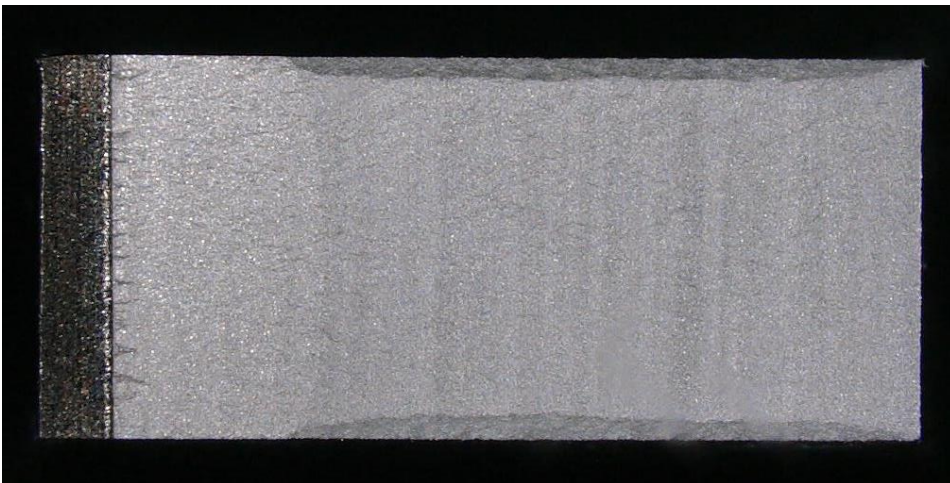
Figure D.49 Optical macrograph of the fracture surface of specimen CP022L.
