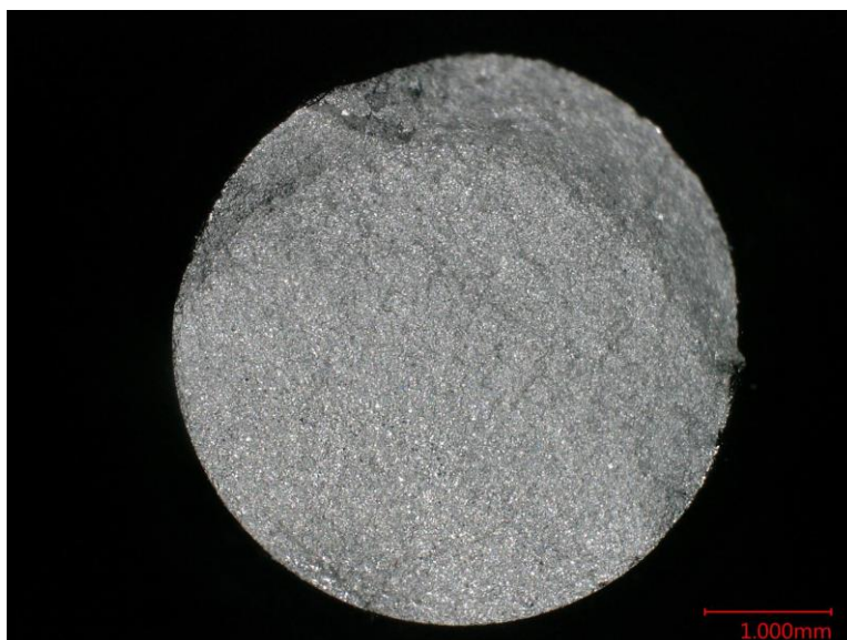
Figure D.8 Optical macrograph of the fracture surface of specimen HF004.
