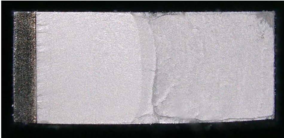
Figure D.48 Optical macrograph of the fracture surface of specimen CP021R.
