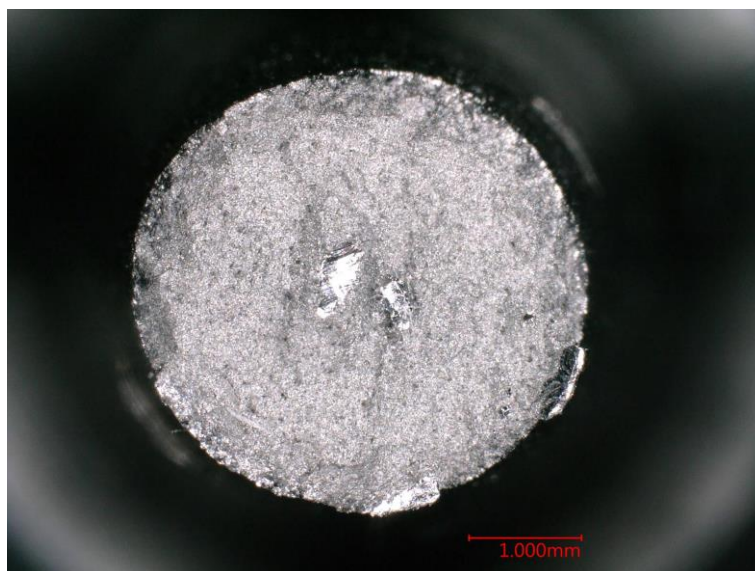
Figure D.4 Optical macrograph of the fracture surface of specimen HT004.
