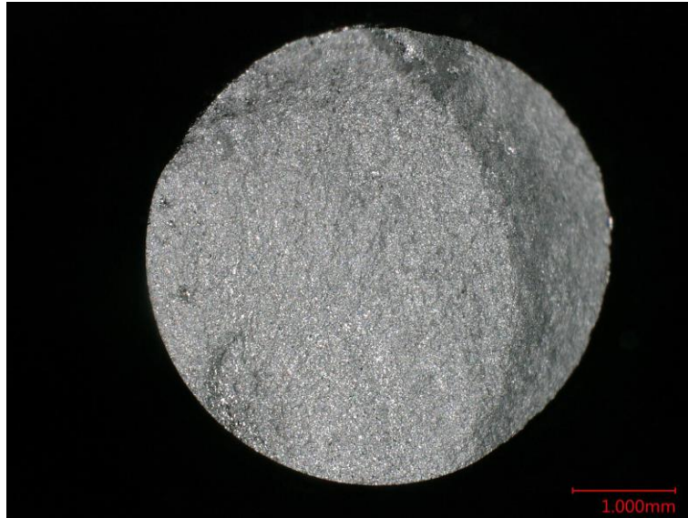
Figure D.19 Optical macrograph of the fracture surface of specimen HF015.
