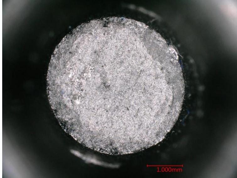
Figure D.1 Optical macrograph of the fracture surface of specimen HT001.
