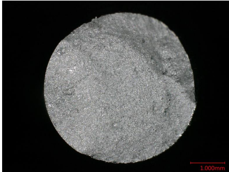
Figure D.21 Optical macrograph of the fracture surface of specimen HF017.
