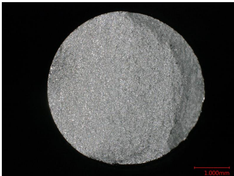
Figure D.7 Optical macrograph of the fracture surface of specimen HF003.
