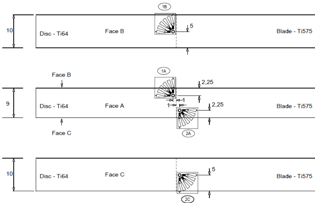
Figure 3.10 Schematic diagram of the location of residual stress measurements. The dashed line denotes the weld interface. (Unit: mm)
