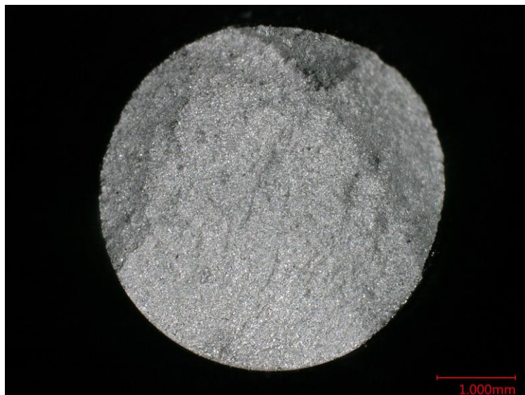
Figure D.22 Optical macrograph of the fracture surface of specimen HF018.
