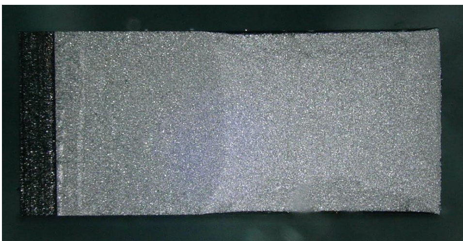
Figure D.50 Optical macrograph of the fracture surface of specimen CP022R.
