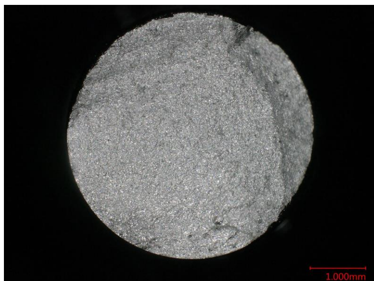
Figure D.10 Optical macrograph of the fracture surface of specimen HF006.
