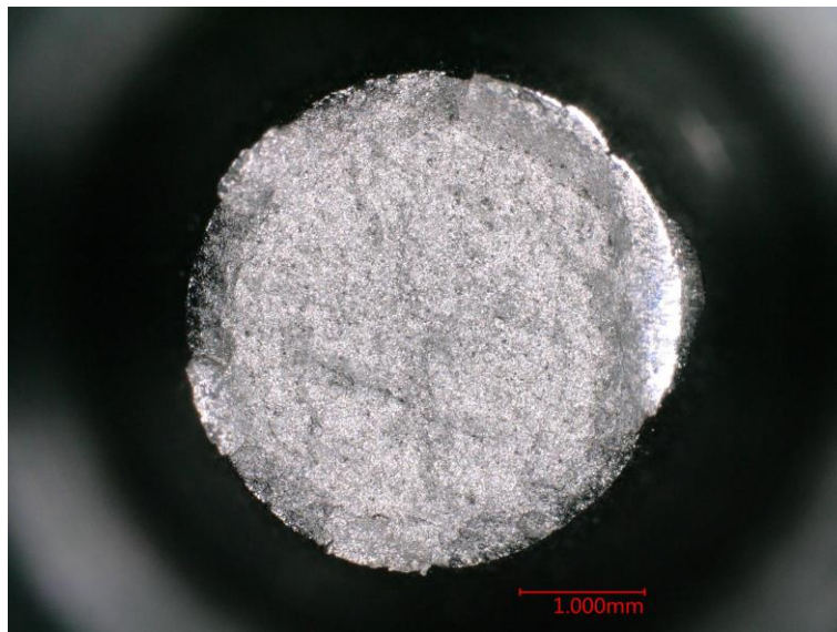
Figure D.2 Optical macrograph of the fracture surface of specimen HT002.
