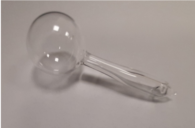
Figure 26: Image showing high pressure vapour cell as delivered. Note the stem is significantly larger than the 20 mm diameter sphere (designed to be \sim 4 mm), also note the imperfect sphere shape causing alignment issues as noted in section VII C
