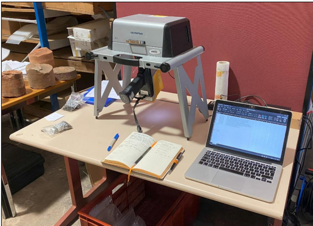
Figure 2.3. Olympus Vanta pXRF workstation set up at GSNI core stores, Belfast, NI
