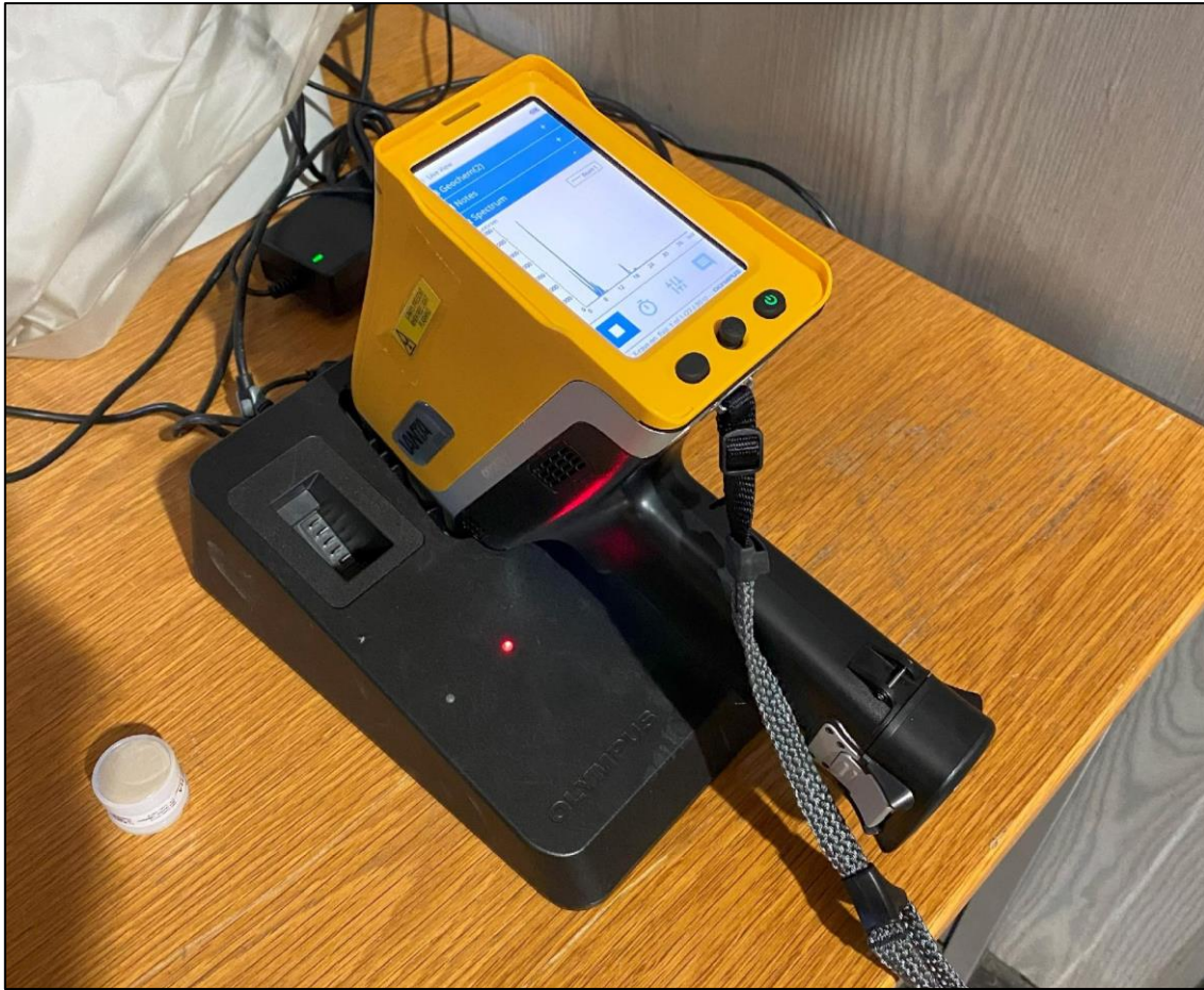
Figure 2.4. Olympus Vanta pXRF unit in charging dock. Analytical Blank and Standard samples to lower left of image
