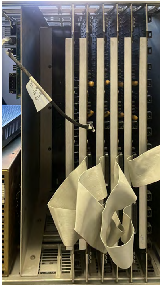
Figure 7.9: ECAT 951 coincidence processor assembly which works very similarly as the ECAT 931 coincidence processor assembly and uses the same backplane. The IPCP cards use a new 80-pin flat ribbon cable to connect to the ACS which also distributes the serial communication between the boards. The updated current loop converter, shown in Figure 7.16, can be seen mounted in the upper left corner of the card cage.
