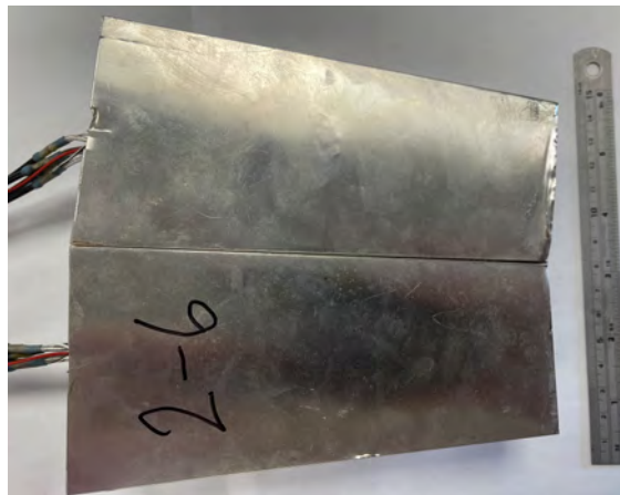
Figure 8.3: SuperPEPT end section EXACT detector block wedge assembly demonstrating the angle of the detector block faces.
