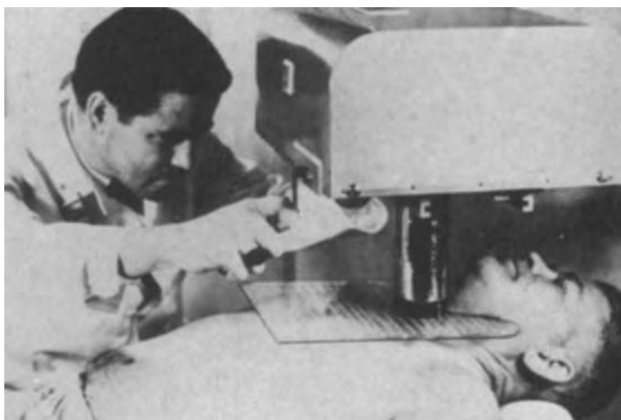
Figure 4.4: An early version of the Rectilinear Scanner used to take a scan of the distribution of ^{131}\text{I} in the thyroid. The scanner is manually positioned by the doctor with the aid of a chart [179].
