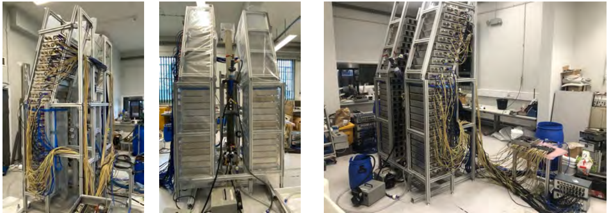
Figure 11.1: View of the custom-built support frame for the LaMA PEPT to surround the FLSmith CoarseAIR TM system in a two-head design [329]. The data, clock, and power cables are visible connected to the modules from the side-views of the system.
