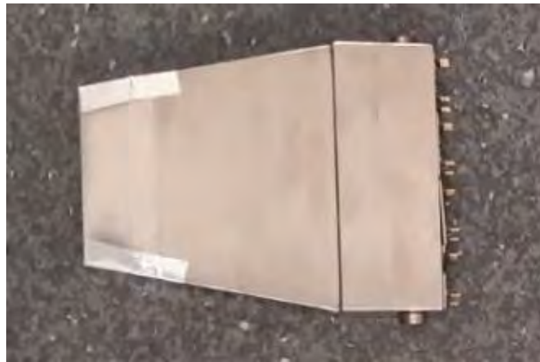
Figure 3. MicroPET cassette as used in constructing MicroPEPT: the four LSO crystals on the left of the picture are connected via light guides to position sensitive PSDs on the right.
