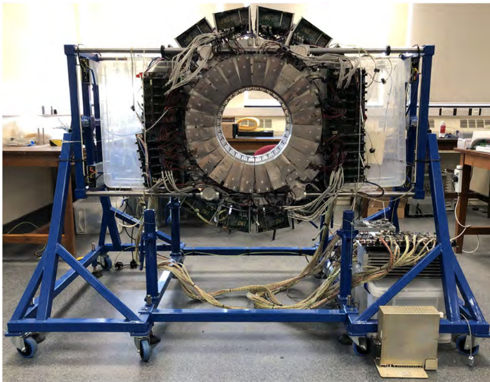
Fig. 3. (Colour on-line) SuperPEPT in its current state of development. The ring assembly is supported by the gantry frame which is able to rotate the central axis of the camera between vertical and horizontal positions (currently in its horizontal position). The data and clock cables running to the coincidence processor and the gantry controller can also be seen; yet to be permanently mounted on the gantry. One of the end sections made up of the EXACT blocks can be seen with its four bucket controller boards on the sides.
