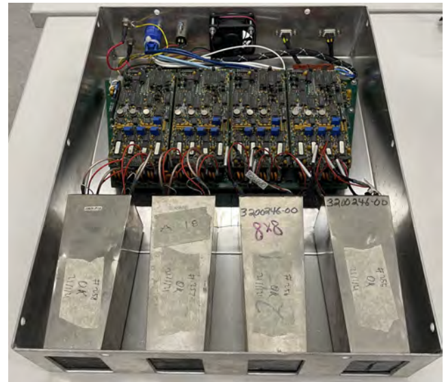
Figure 2: A LaMA bucket with its lid removed displaying four detector blocks and a bucket controller board from the ECAT 951 PET scanner.
