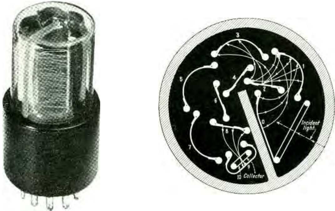
Figure 3.16: The electrostatically focused photomultiplier tube designed by Rajchman of RCA. The design is more compact than that of the original multi-stage PMT with increased gain [88].
