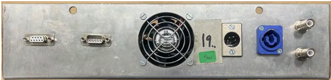
Figure 9.4: A view of the connectors available on the back side of the LaMA bucket. From left to right: female DB-9 connector for the differential ECL clock and serial communication line, male DB-9 connector for the differential ECL data connection to the coincidence processor, a cooling fan, male 4-pin XLR for 12 VDC supply for the fan, female Neutrik powerCON socket for a logic 5 VDC, -5.2 VDC, and common ground, and two SVH 1.5 kVDC sockets for daisy-chaining the HV supply through all the buckets.
