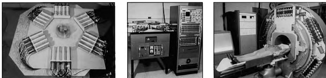
Figure 4.34: (Left) The PETT II system built at EG&G ORTEC and used for obtaining test data used to establish the principles of PET. (Centre) The PETT II 1/2 system which was identical to PETT II but featured a computerised platform used for positioning phantoms and small animals. (Right) The PETT III/PET III or a full-sized version of PETT II was built at Washington University with double the amount of detectors that were able to produce the first quantitative results in human PET scans [244].
