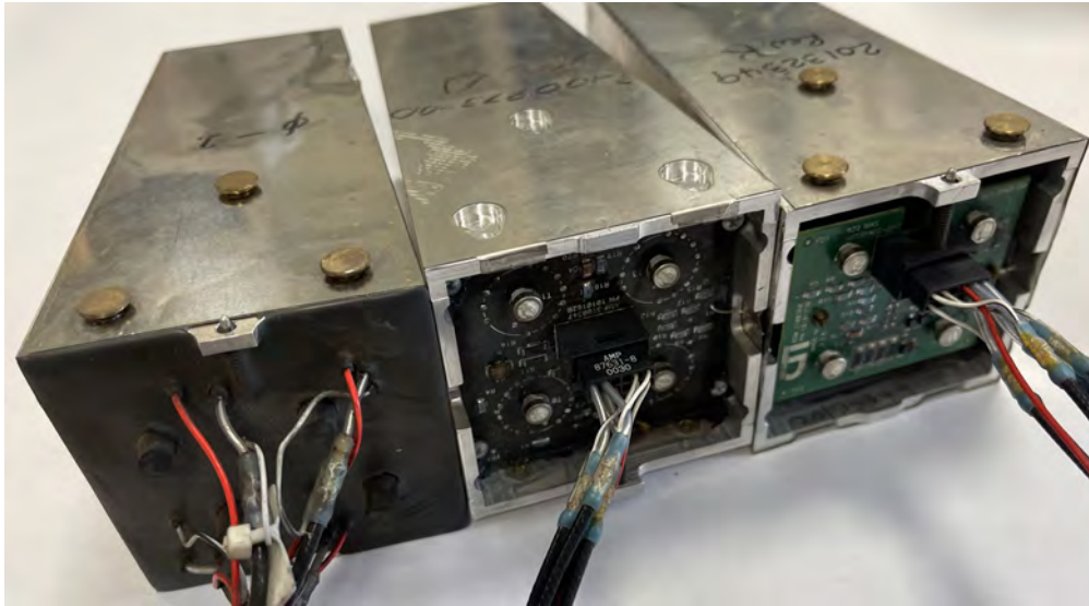
Figure 6.3: The evolution of the HV and signal distribution board in the ECAT EXACT series of detector blocks. Left to right: An early detector block design with a fully potted board. A detector block with an exposed board and removable leads. The latest ECAT EXACT detector block with a removable board and leads.
