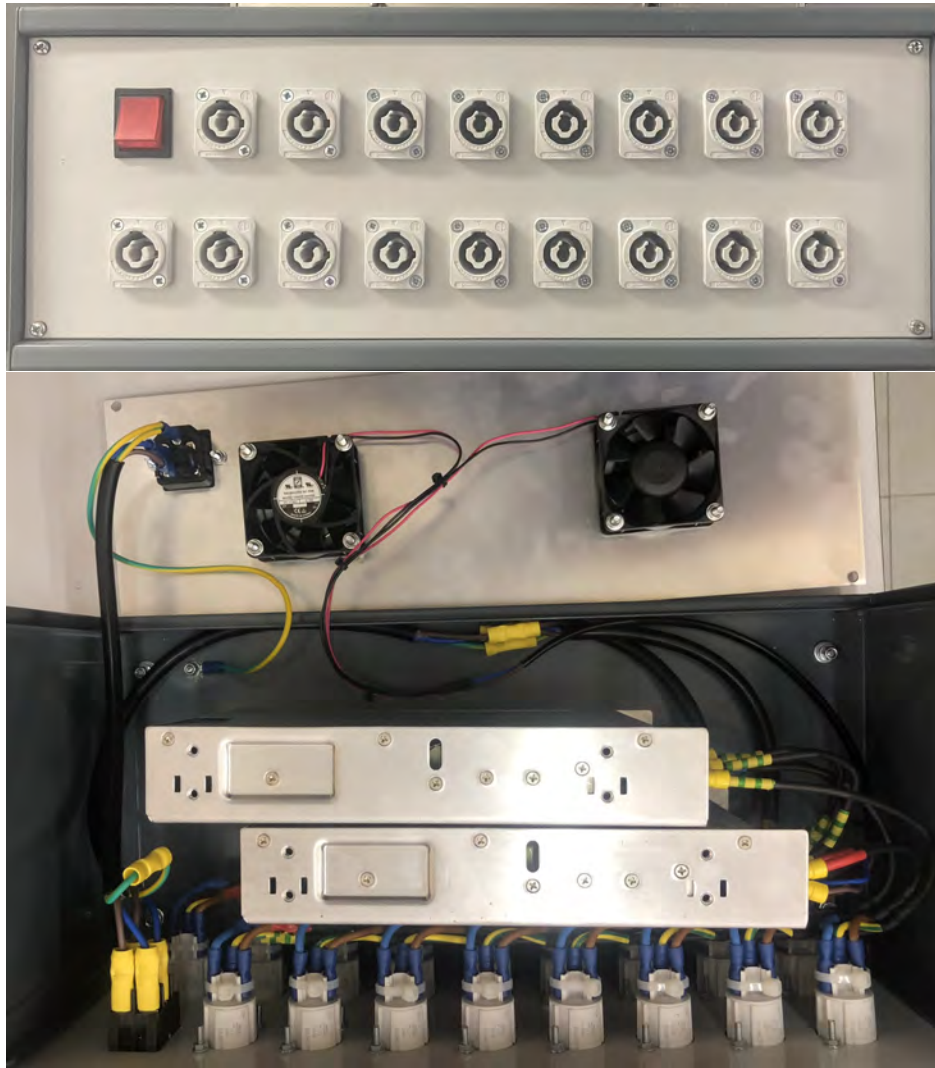
Figure 9.2: New logic power supplies for the LaMA PEPT. This is 1 of 3 modules made with each one being able to support 17 connections or 16 modules and 1 spare. The system uses commercial, heavy-duty Neutrik powerCON connectors with internal power distribution utilising solid copper conductors.
