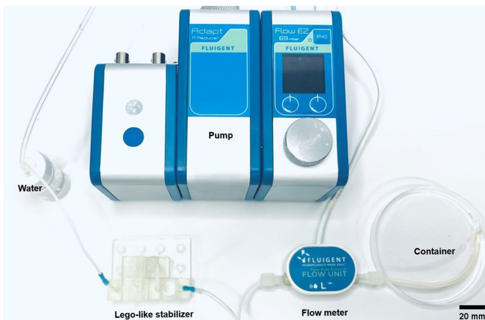
Fig. 5-4 The experimental set-up for extracting stabilisation ratios and RC constants of different levels of stabilisers.
