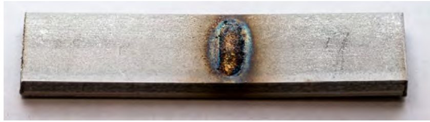
FIGURE 2.30: Residual deformations produced by a metal deposition process, usually called angular distortion in welding. Image reproduced from [150].
