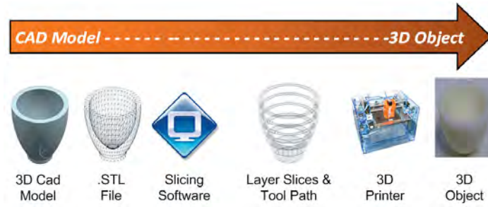
FIGURE 2.2: Necessary procedural steps for the additive manufacturing process, from the digital CAD model to the final 3D object. Image reproduced from [13, p. 3, fig. 1].
