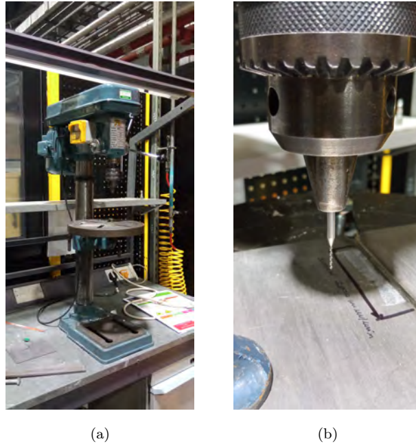
FIGURE 4.4: Pillar drilling machine on the left (a) and a detail with the Ti-6Al-4V plate on the right (b).
