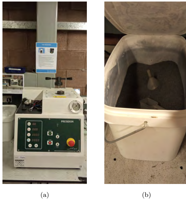
FIGURE 4.7: Hot mounting machine on the left (a) and the Bakelite powder on the right (b) used to embed the specimens.
