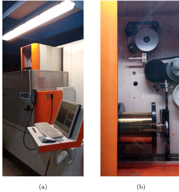
FIGURE 4.6: Electric Discharge Machine on the left (a) and a detail of the metallic wire spool on the right (b).
