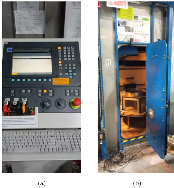
FIGURE 4.5: Control panel of the Trumpf ® machine on the left (a) and entrance of the chamber on the right (b).
