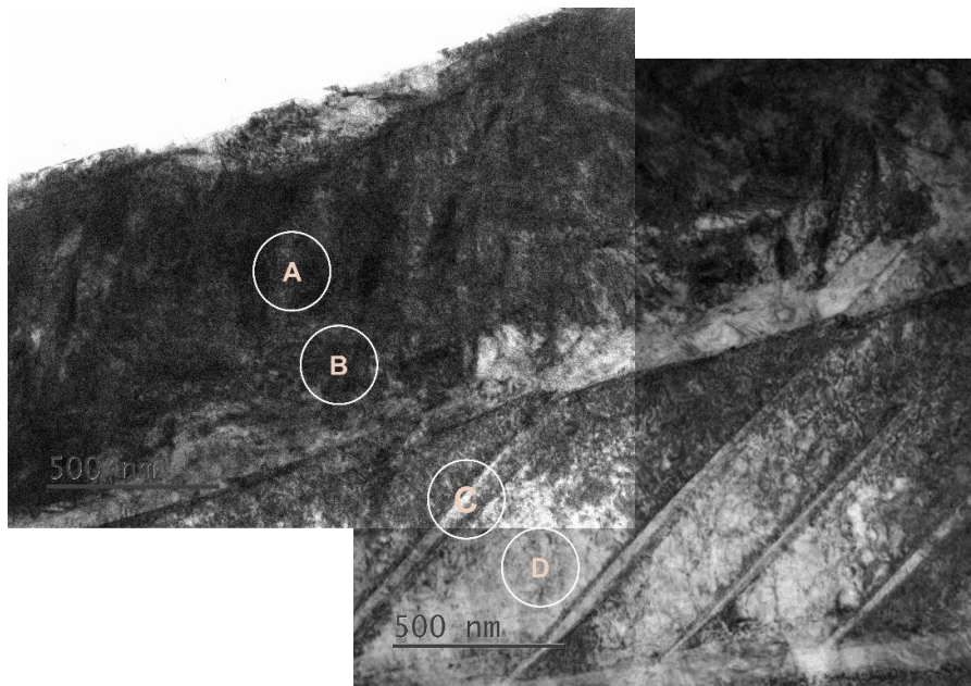
Figure 57: SAED patterns taken from the 3-Shock surface close to the imaging condition of the matrix BD = 1\bar{1}01 . A) shows the diffraction in a surface twin array with B) showing a similar location also covering regions outside the twin array. C) Depicts the diffraction pattern of the matrix and a thin twin (also seen in Figure 54) whilst D) shows the zone axis pattern within the matrix.
