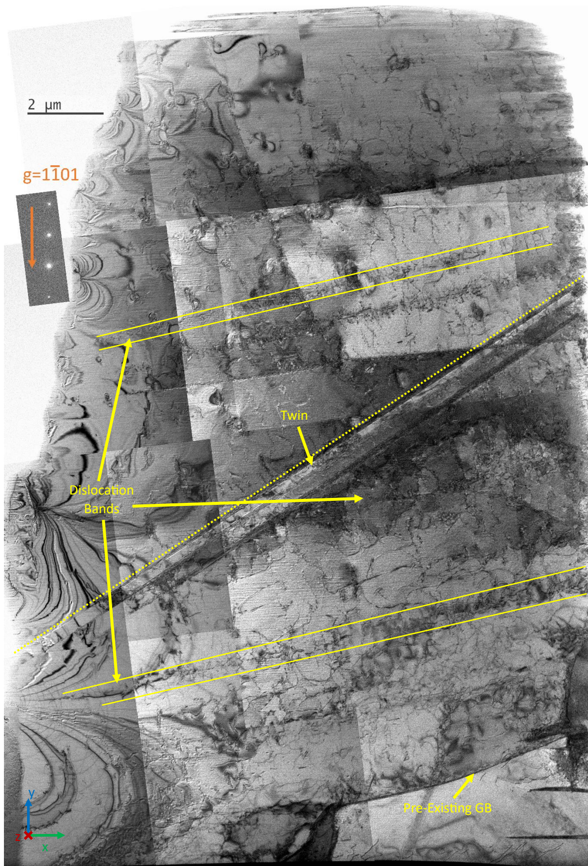
Figure 71: 15-Shock TEM sample taken 250 \mu\text{m} from the shock surface parallel to this surface. Imaged using g = 1\bar{1}01 . Further analysis can be seen in Figure 110. Dislocation bands are labelled non-exhaustively.
