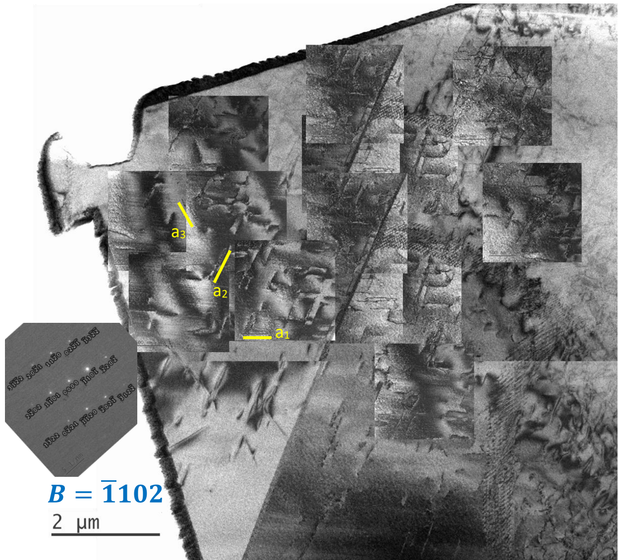
Figure 88: 3-Shock TEM sample displaying Dislocation lines. Imaging condition B = \bar{1}102 (at zone axis). This serves as the background to Figure 89, Figure 90, Figure 91, Figure 92 and Figure 93 for locational accuracy. These are all near B \cong \bar{1}102 .
