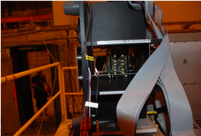
Figure 7.5: A picture of the completed TPAC 1.2 sensor stack. Once placed in the test beam the stack was positioned so that the base of the stack (on the left hand side of this picture) faced the test beam, with the beam passing through the centre of the stack. This picture shows that the sensor PCB which would be hit second and the sensor PCB which would be hit sixth by test beam particles are inverted relative to the other sensor PCBs. These two sensor PCBs were inverted so that they could be placed in slots adjacent to the sensors first and fifth in line for the test beam without interfering with their cabling. For the same reason the sensor PCBs third and forth in line for the test beam (the test sensors) are rotated ninety degrees relative to all the other sensor PCBs (the control sensors).
