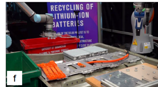
Step 3: Sorting, using VG10 suction gripper to pick and place the cover in the waste
