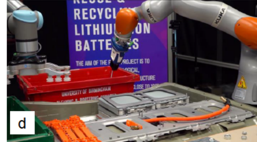
Step 2: Sorting, grasping bolts with 2 finger gripper and place in the waste basket
