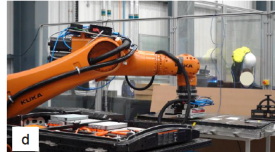
c) Using vacuum gripper to pick modules and d) sort them with Kuka KR500
