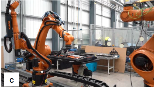
c) Using vacuum gripper to pick modules and d) sort them with Kuka KR500
