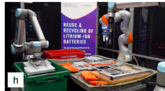
Step 4: Sorting, using VG10 gripper to pick and place modules in the recycle bin
