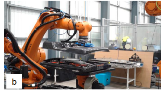
a) Using vacuum gripper to pick the lid of battery pack and b) remove it with Kuka KR500
