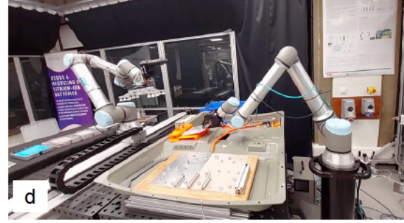
c) Dual arm collaboration to grasp a cell and d) place it on the Testbed.
