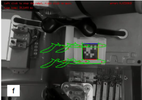
e) Using the modified HDVS to track a dynamic module f) Image screen and trajectory (green)
