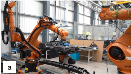
a) Using vacuum gripper to pick the lid of battery pack and b) remove it with Kuka KR500
