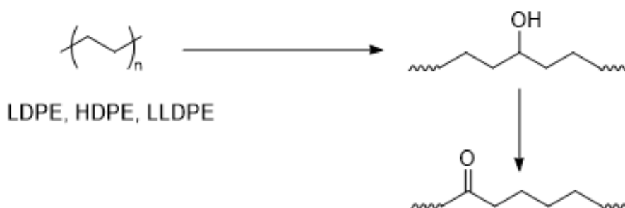
Scheme 1.2 General scheme for the hydroxylation of polyethylene followed by secondary oxidation
