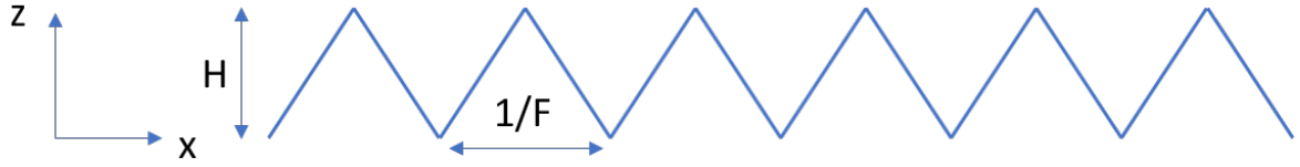
Figure 5.1: 2D geometry of interface required for a prismatic morphology, where H is the height of the peaks and F is the frequency of the peak per mm.
