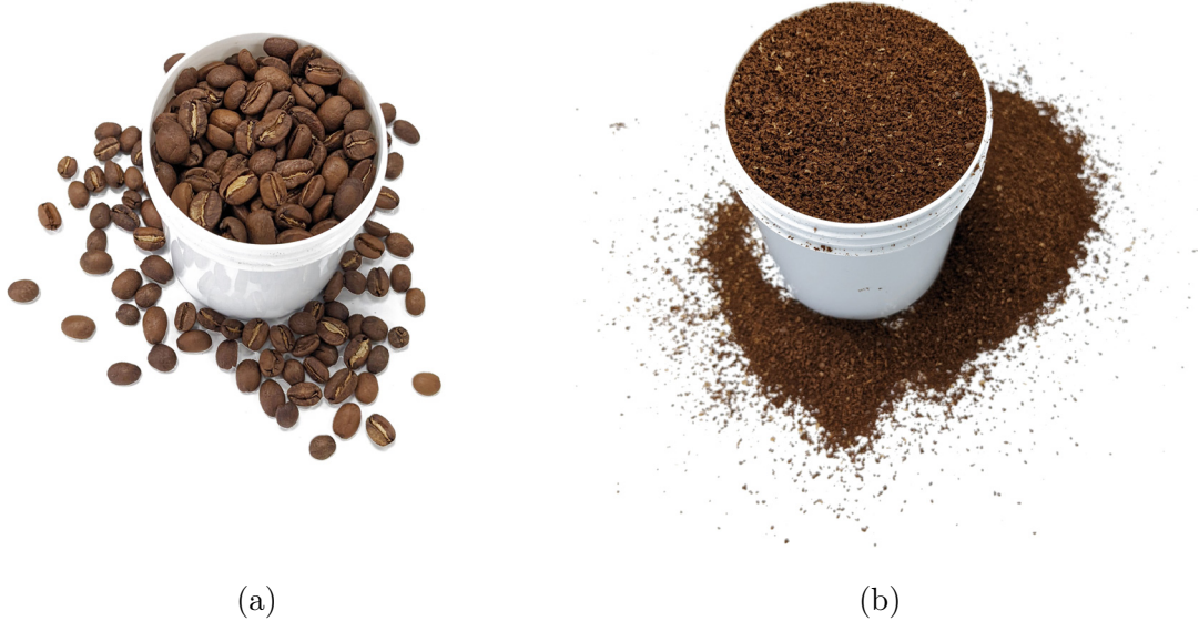
Figure 3.4: Measurement of (a) whole bean and (b) ground coffee bulk density using a free-settling method.
