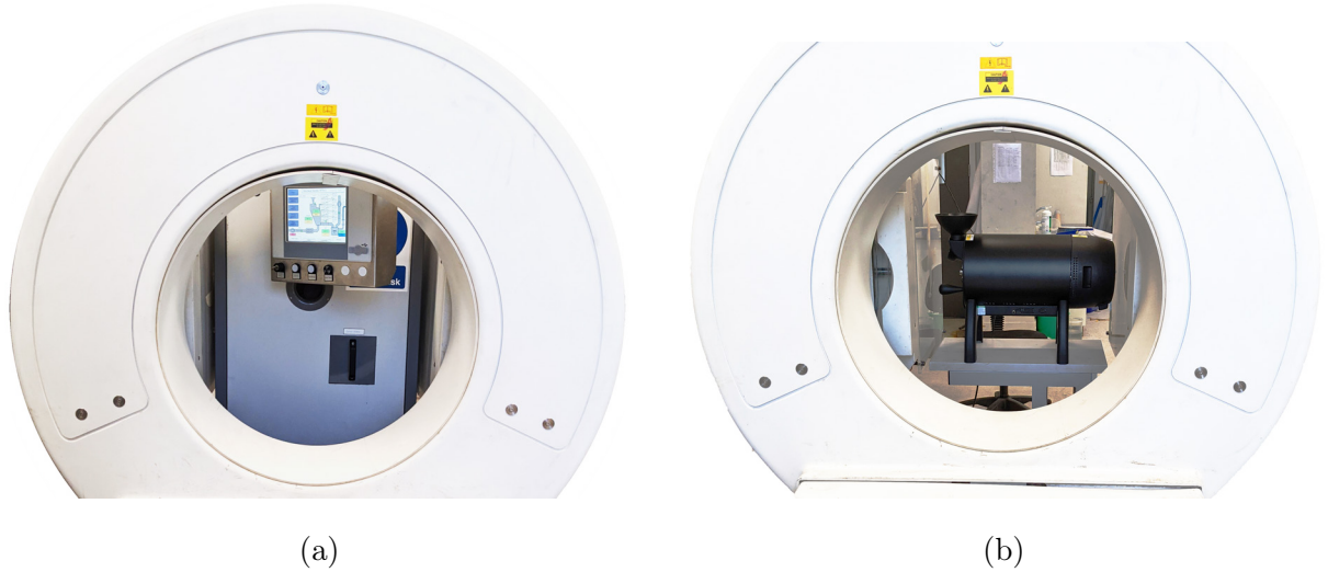
Figure 4.2: Photographs of the (a) spouted bed and (b) rotating drum roasters, used for flow studies, positioned in the ADAC Forte positron camera.
