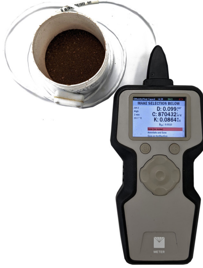
Figure 3.8: Measurement of the thermal properties of ground coffee samples using a thermal properties analyser (TEMPOS, METER Group).
