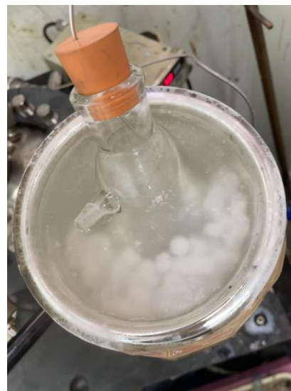
Figure 5-5: Acetone and dry ice regulated solvent trap, containing acetone and artificial electrolyte.
