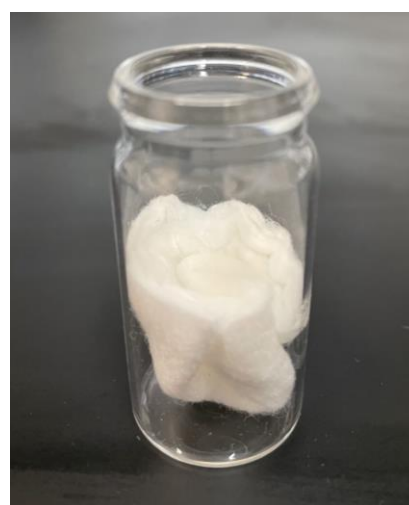
Figure 5-4: Glass sample holder containing electrolyte components absorbed in a cotton wool matrix.
