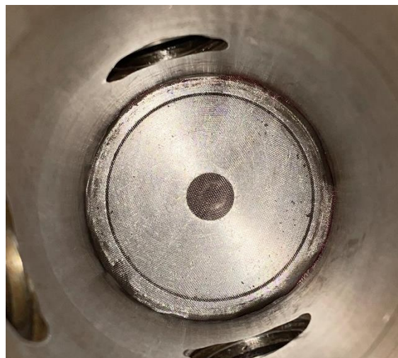
Figure 6-2: Photograph of HPV internal body, with steel mesh filter resting on base.
