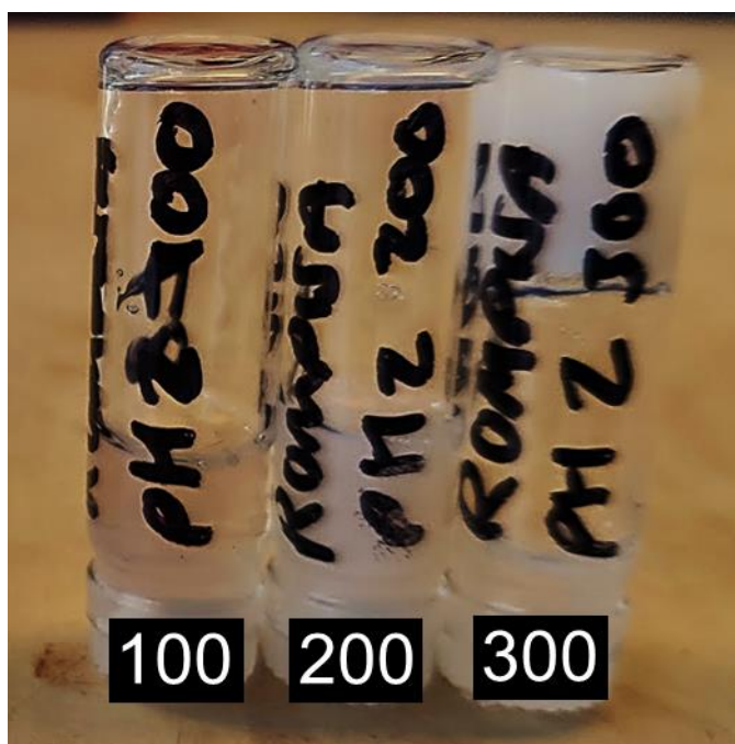
Figure S2.3. Inverted vial test of P pH2 1 x , from left to right x = 100, 200 and 300.
