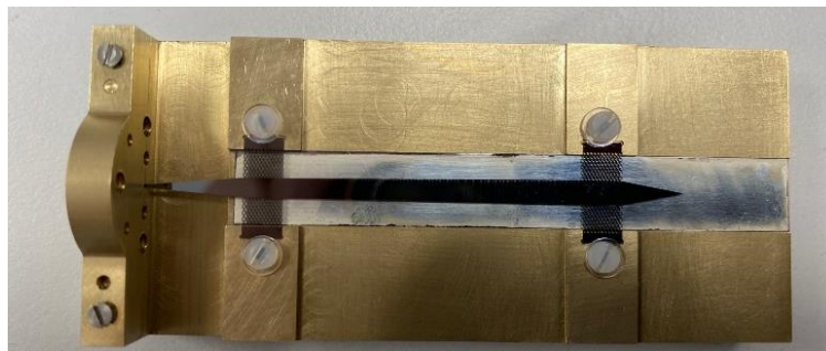
Figure 4.21. The assembled DLWA is formed from a micromachined HRS piece suspended above a reflector. A UG387/U waveguide flange (left side of the photo) is used to interface with a WR-3 rectangular metal waveguide which excites the HRS DSW.
