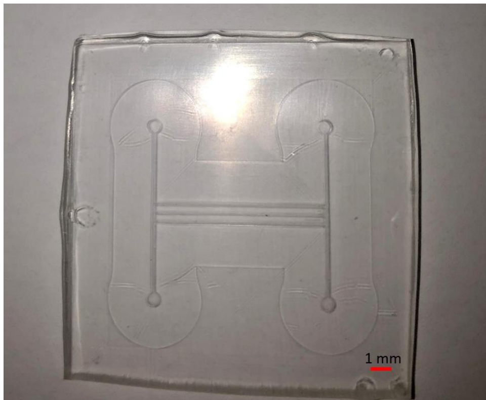
Figure 5.3: Micro milled PMMA microfluidic device. Average channel width and height is 300 \mu\text{m} , gate restriction dimensions are 30 \mu\text{m} x 10 \mu\text{m} .
