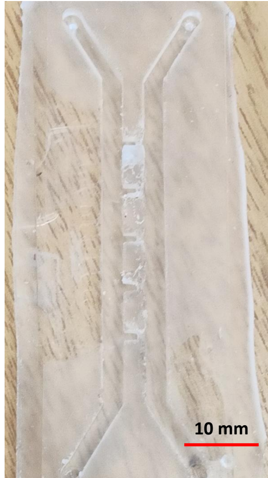
Figure 3.7: Replicated structure of the 3D printed mould for gates in the bottom position with thermal curing at 25 °C for 24 hours. The top of the device thickness is 5 mm.
