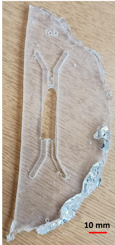
Figure 3.6: Rupture across the channel centre for the top gate design with the 45 minute at 100°C thermal curing method for the PDMS. The top of the device thickness is 2 mm.
