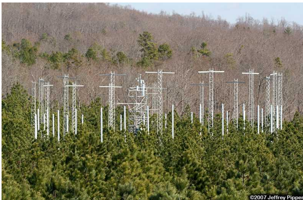
Figure 10: Duke FACE. Tree fertilisation experiment, showing adjustable vent pipes and supporting towers (Pippen, 2007).
