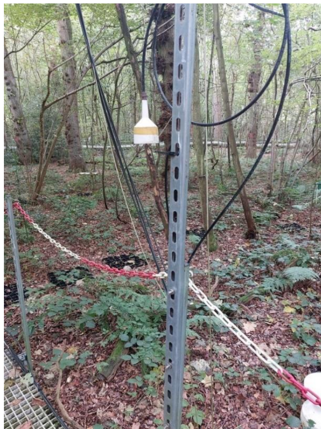
Figure 18: Example of one of the inlet funnels and pipe at 2 metres high.
