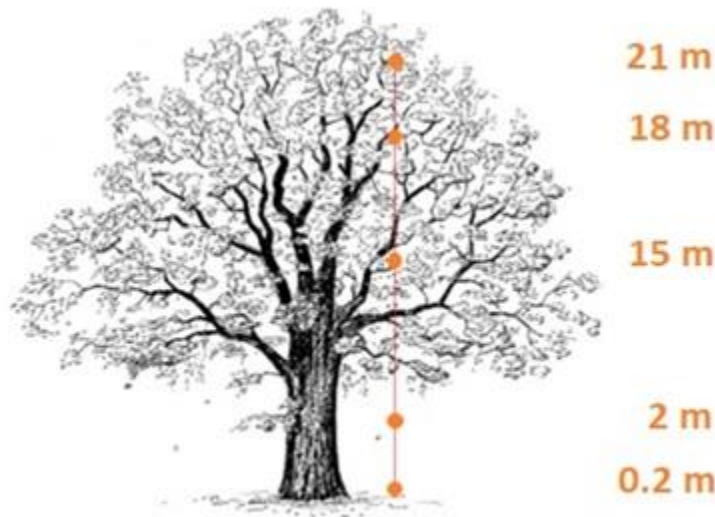
Figure 3: Air sampling points. The typical arrangement of the air sampling inlet ports suspended from a tree branch closest to the centre of the research space. Image adapted from (Mateusz, n.d.).
