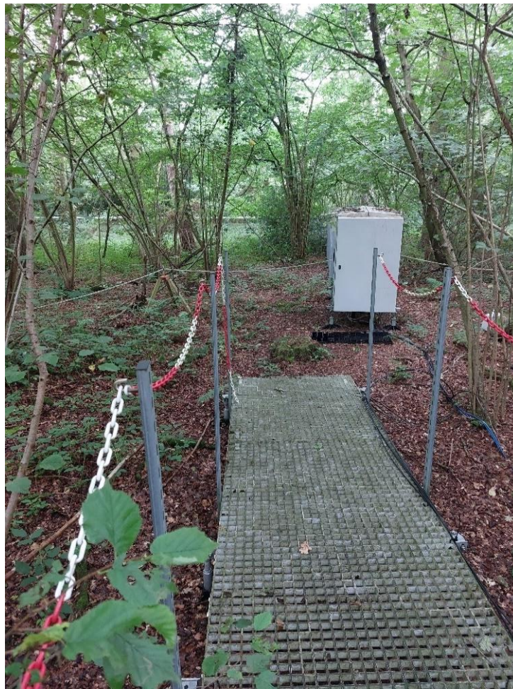
Figure 15: Typical installation of the monitoring cabinet. The cabinet is mounted just outside of the experimental space; this is the cabinet at space 9 (see to figure 1 for a location map of the site).
