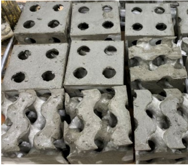
Figure 8.1 Concrete Primitive and Gyroid TPMS structures from [197].
