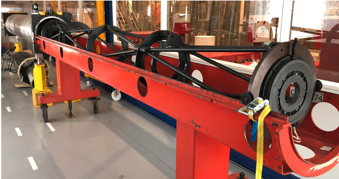
Figure 3.6: Image of an opened CEDAR, photograph taken by Serge Mathot (CERN). The mechanical frame holding the diaphragm, Mangin Mirror and Chromatic Corrector on the optical axis is visible.
