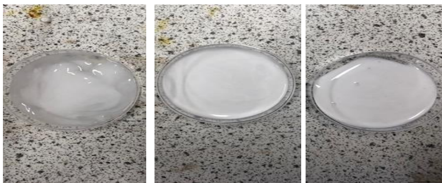
Figure 4.5: (L – R): Sample D (7.5% Wax, 5% Surfactant)– White, very viscous and translucent, Sample E (10% Wax, 5% Surfactant) – Milky Consistency, runny and very pourable, Sample F (15% Wax, 5% Surfactant)– White, Milky and Very easy to pour.
