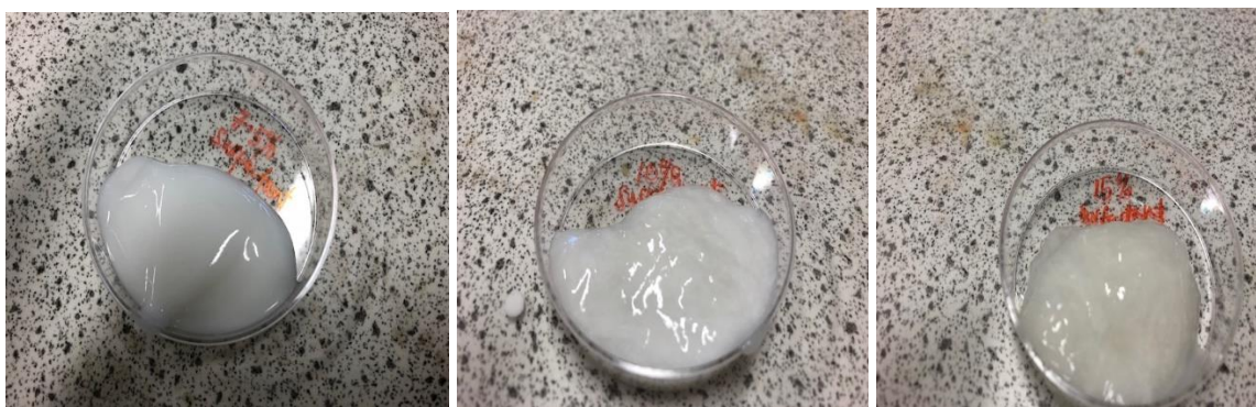
Figure 4.1: (L – R): Sample A – White, soft-gel like material and not resistant to flow, Sample B – Off-white, lumpy gel and slightly pourable, Sample C – Off-white, Lumpy and Resistant to flow.
