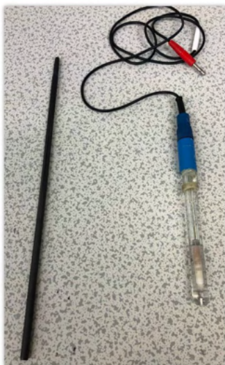
Figure 3.1: Graphite rod counter (left) and saturated silver/silver chloride reference electrodes (right) used for ex situ corrosion testing.
