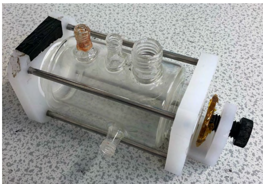
Figure 3.2: Electrochemical cell used for ex situ corrosion testing.
