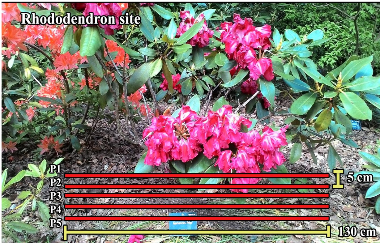
Figure 57. The GPR survey setup with details about profiles with the 4 GHz antenna.
