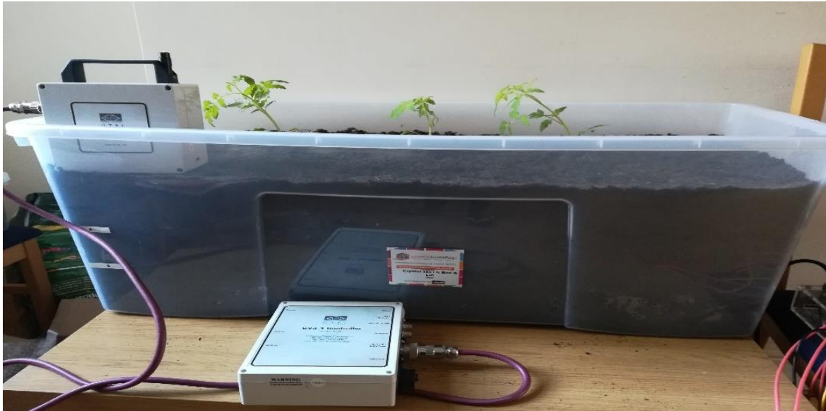
Figure 69. Example of GPR survey using the 4 GHz antenna in the large container with 3 tomato plants.
