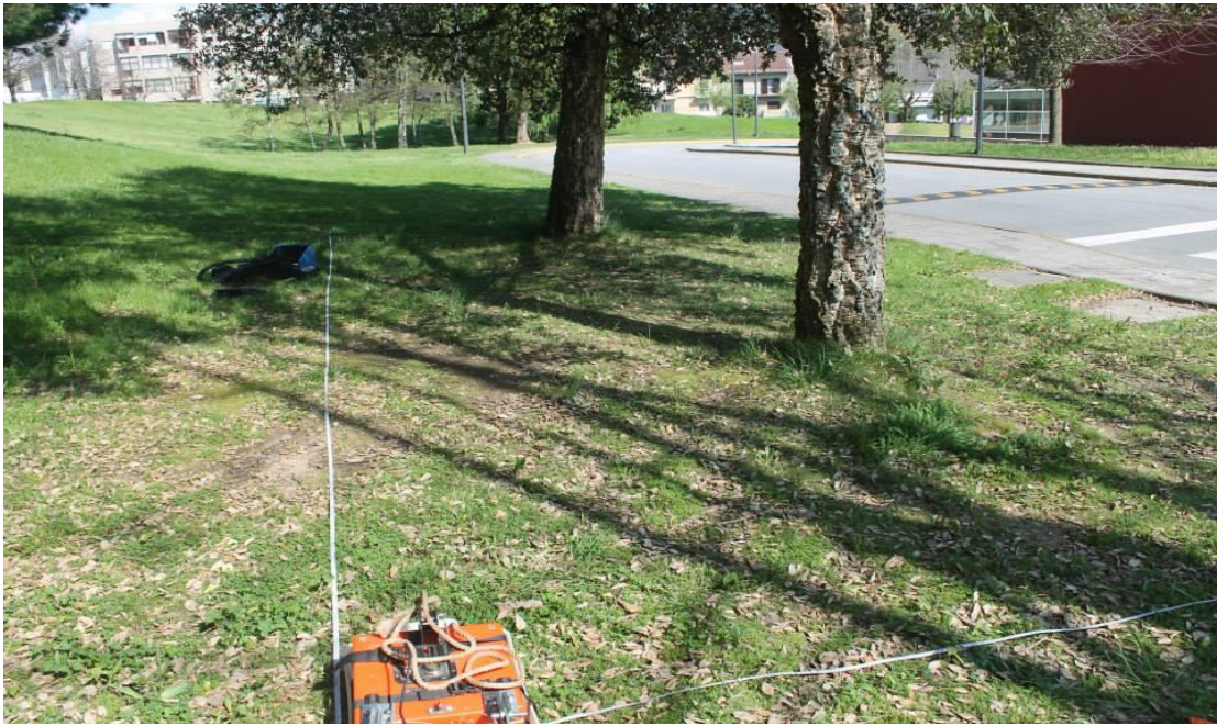
Figure 5. Planning the survey grid using measuring tapes, with a 400MHz antenna.
