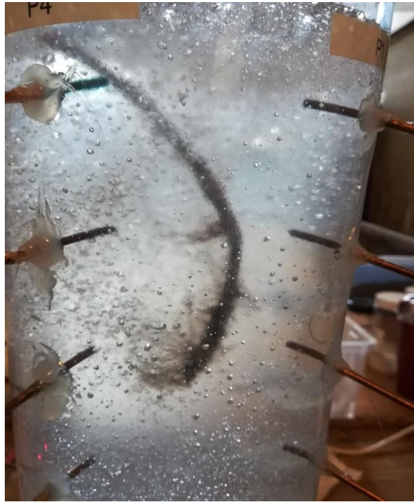
Figure 27. Example of a plant immersed in a transparent soil type created by grounding KI-gel 201KA aquabeads granules. This represents the type of soil used in the case study which will be presented at the methodology section.
