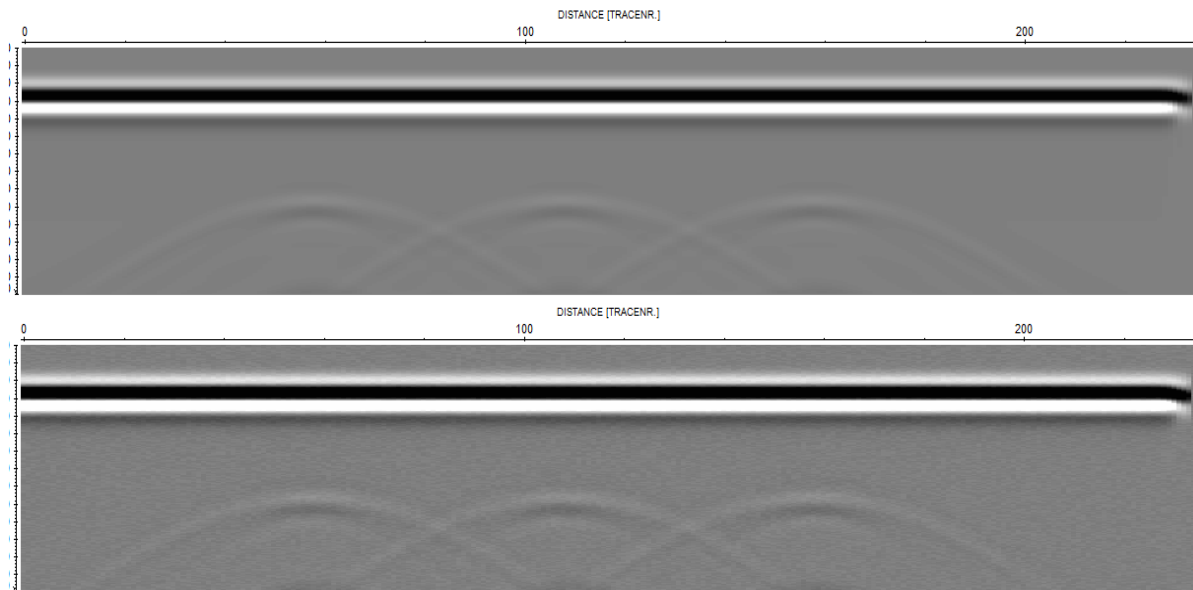
Figure 82. Model F - a GPR model consisting of a soil unit with a permittivity value of 17.77 and root permittivity value of 15. Model created with the 1.5 GHz antenna.
