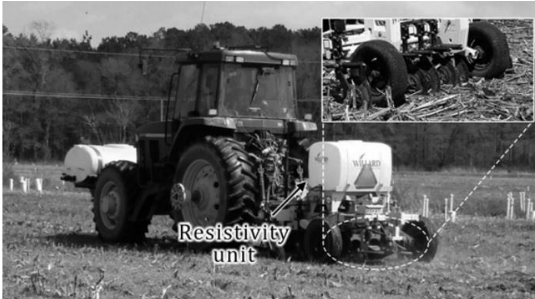
Figure 28. Image showing an example of a resistivity equipment using disks as electrodes developed by Veris Technologies (Binley and Slater, 2020)
