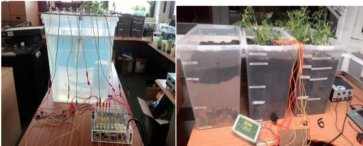
Figure 1 Left – three of the test boxes with tomato plants; the box in the middle has one plant and the one on the right has three plants. Right – one of the boxes with one tomato plant, water and fertilizers. In both images, part of the equipment can be seen, the resistance meter (left) and the switch box (right).
