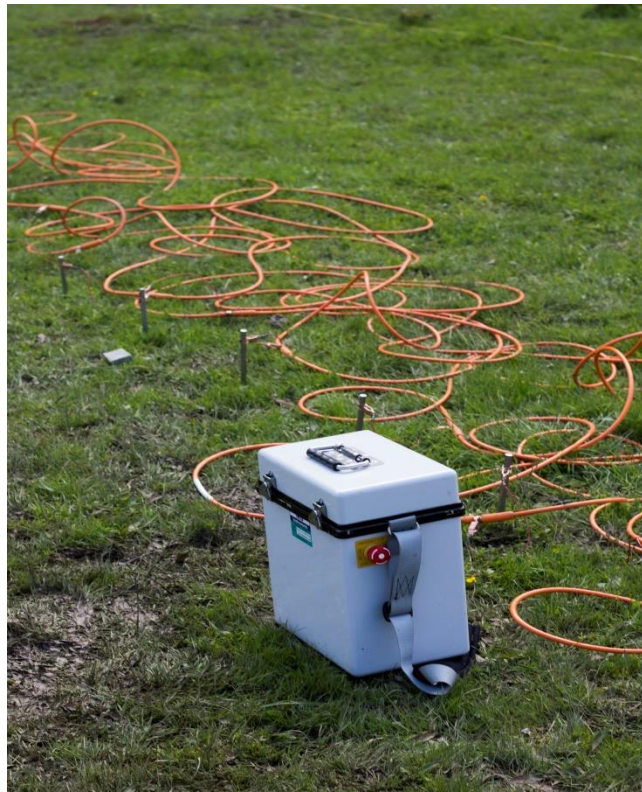
Figure 16. Example of a survey using multielectrode equipment, which requires all the electrodes to be inserted into the ground at the same time, while the equipment automatically carries out the survey.
