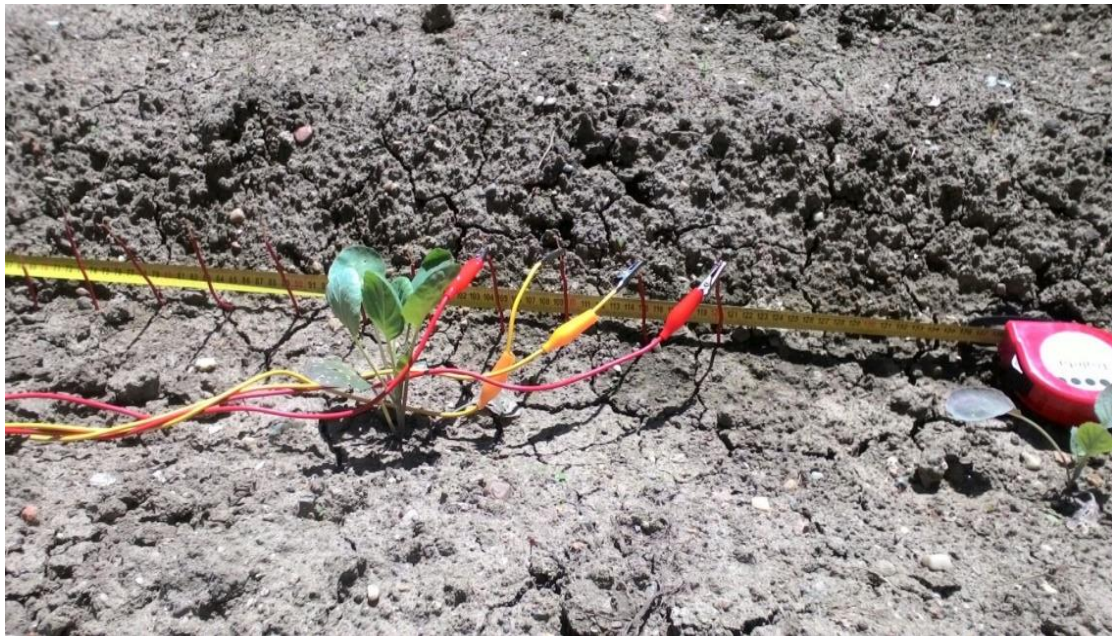
Figure 85. Image showing surveying with the resistivity method in a young cabbage field.
