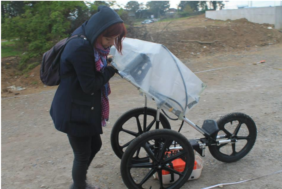
Figure 3. Example of a survey using a 400MHz antenna and a cart with 3 wheels. The console is covered with a plastic foil for protecting the console from rain.
