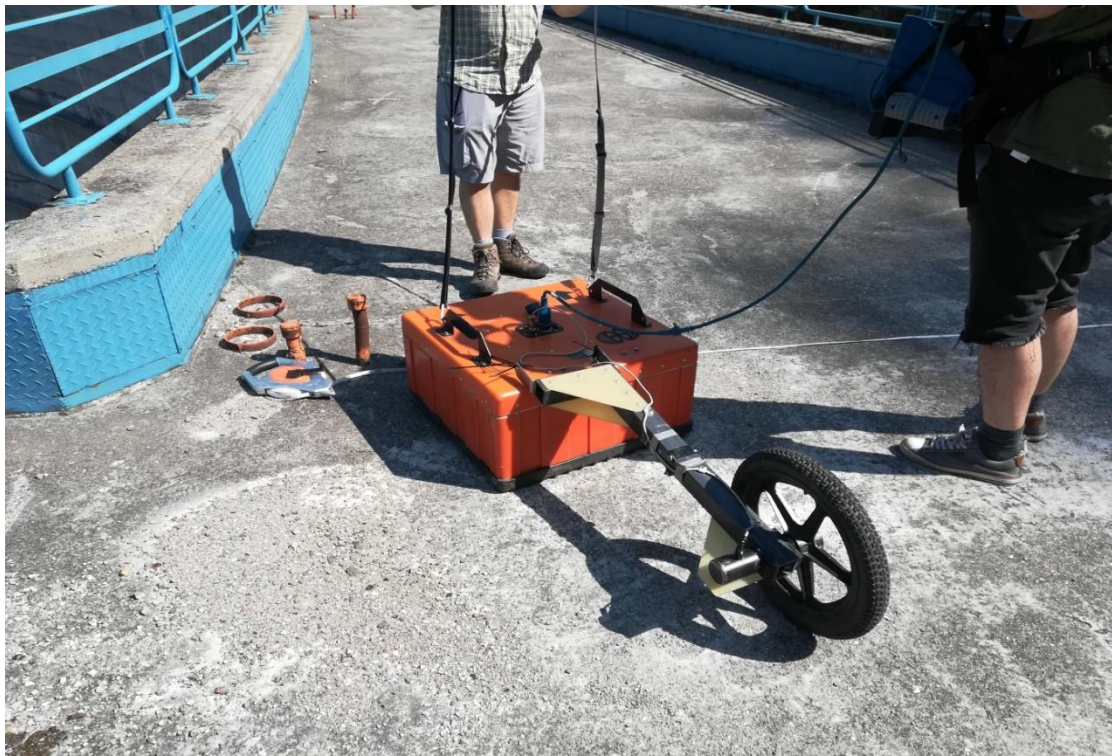
Figure 4. Example of a survey using a 200MHz antenna and a single wheel. One person drags the antenna and the other is controlling the console.
