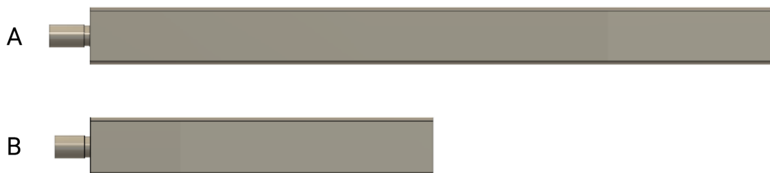
Figure 2.2: Models of titanium paddles manufactured to act as cell incubation substrates and designed to attach to transducer (sonotrodes) for oscillation at 20 (A) and 40 kHz (B). 20 and 40 kHz strips are 118 and 57.5 mm respectively excluding the screw.
