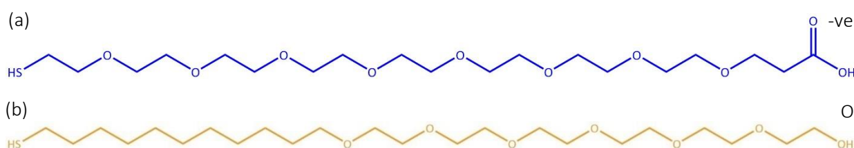
Figure 8.2 Structure of PEGylated thiols used to functionalise PtNPs. (a) O-(2-carboxyethyl)-O'-(2-mercaptoethyl) heptaethylene glycol (2-MOHA) and (b) 11-mercaptoundecyl)hexa(ethylene glycol) (11-MUHEG).
