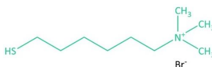
Figure 6.7 Structure of (6-mercaptohexyl)trimethylammonium bromide (6-MTAB).
