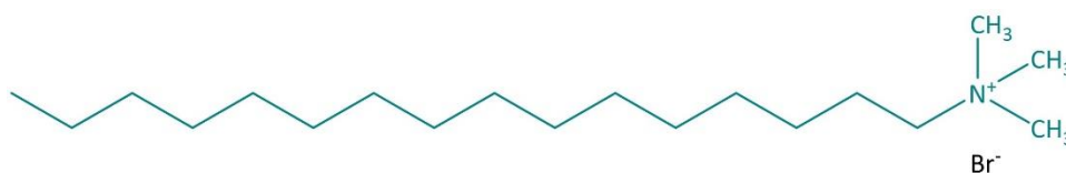
Figure 6.4 Structure of cetyltrimethylammonium bromide (CTAB).
