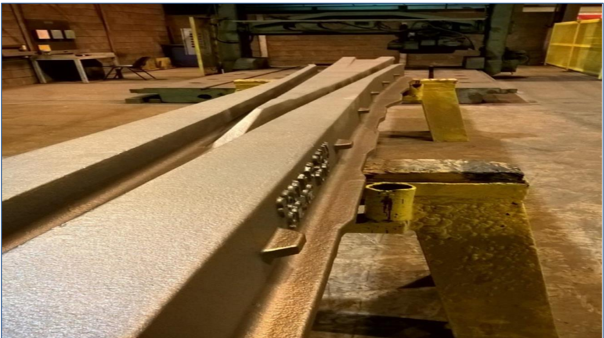
Figure 21: NR60 MK2 Cast Crossing at S&C Manufacturer's Yard (Network Rail, 2016)
