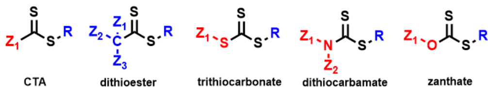
Figure 1.2. Typical structures of chain transfer agents (CTAs) based on the functionality of the Z- group. Reproduced from ref. 42
