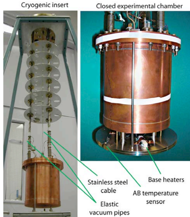
Figure 4.14: Photos showing the cryogenic insert and the closed experimental chamber.
