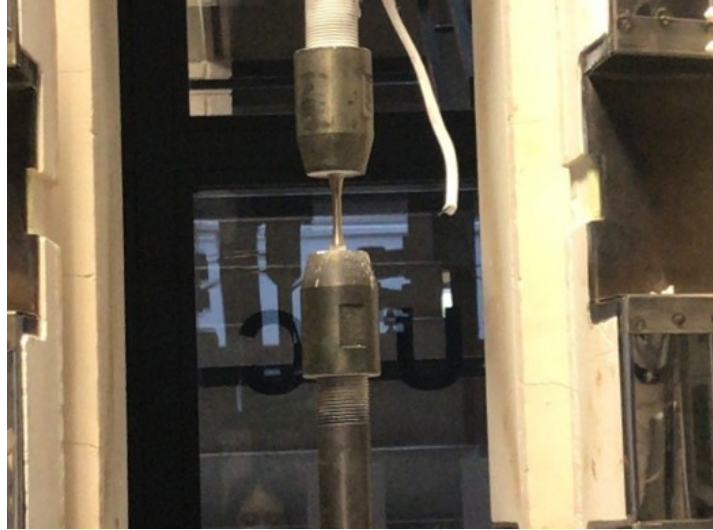
Figure 3-17 HT sample installed on ESH hydraulic testing machine
