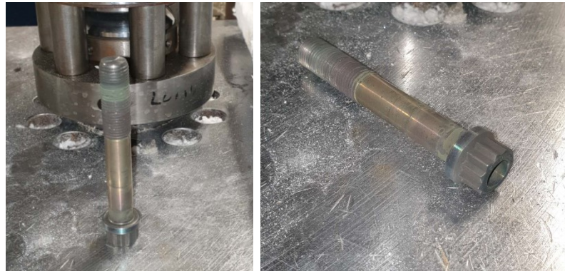
Figure 3-12 Group C IN718 large bolt installed in the testing machine by the customised fixture in the middle
