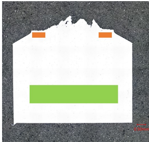
Figure 4-56 Demonstration of the microhardness test applied on cross-sectional microstructure of sample HT2
