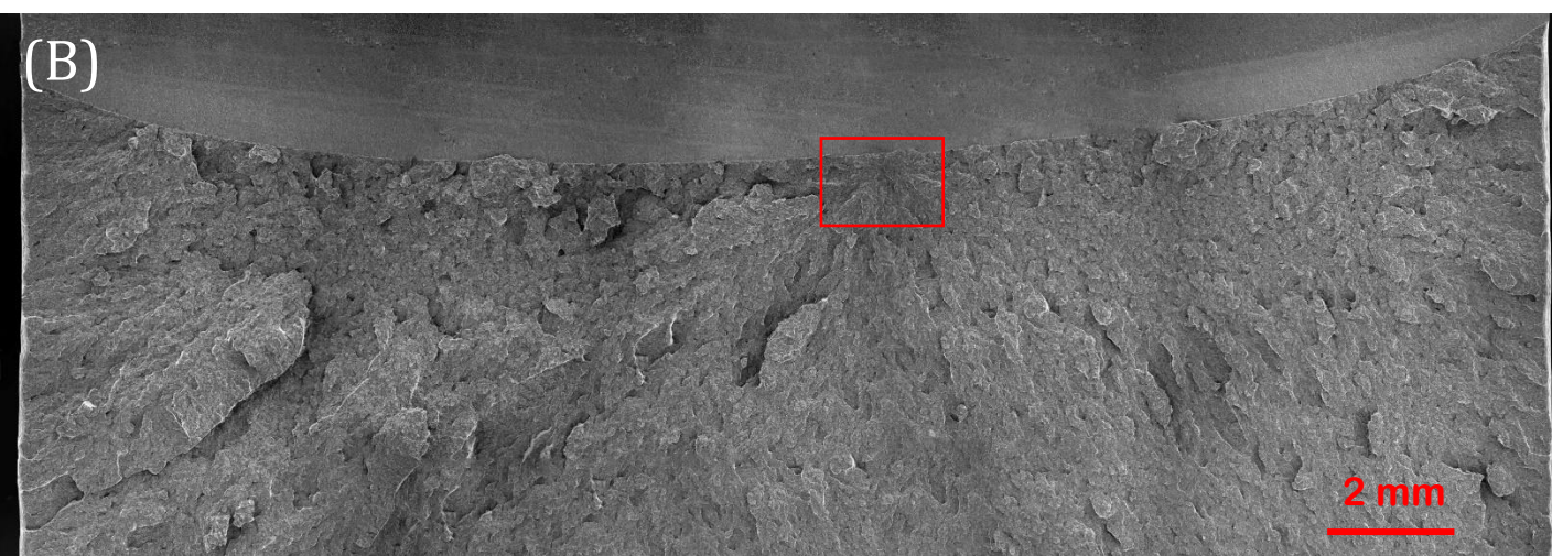
Figure 6-20 (a). Overview of fracture surfaces on a sharp-cracked specimen, designated CT HT2-05, tested at -120\text{ }^{\circ}\text{C} . Red frames on matching halves (A) and (B) denote the most probable fracture initiation areas. Test results: Critical J-integral ( J_c ) value of 23.9\text{ kJ}/\text{m}^2 , crack tip opening displacement (CTOD) of 0.018\text{ mm} , local cleavage fracture stress of 1986\text{ MPa} ( n=0.1 ), fracture initiation distance ( X_o ) of 256\text{ }\mu\text{m} , and an average stable crack extension of 10\text{ }\mu\text{m} .
