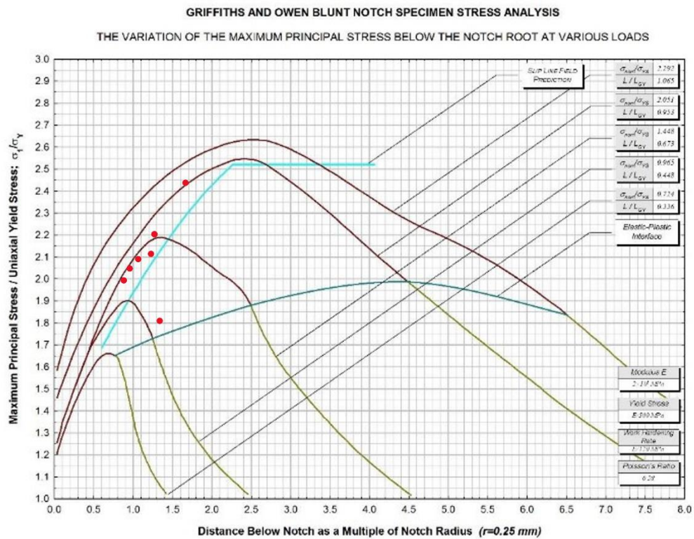
Figure 6-50. Initiation Site Locations in relation to FEM Stress Distribution. (the seven red dots represent the result of each test)
