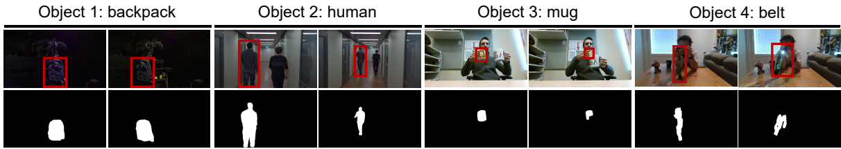
Figure 3.11: Qualitative results of our pseudo label generation network during inference. Our approach can effectively convert the bounding boxes to masks with effective RGBD fusion.
