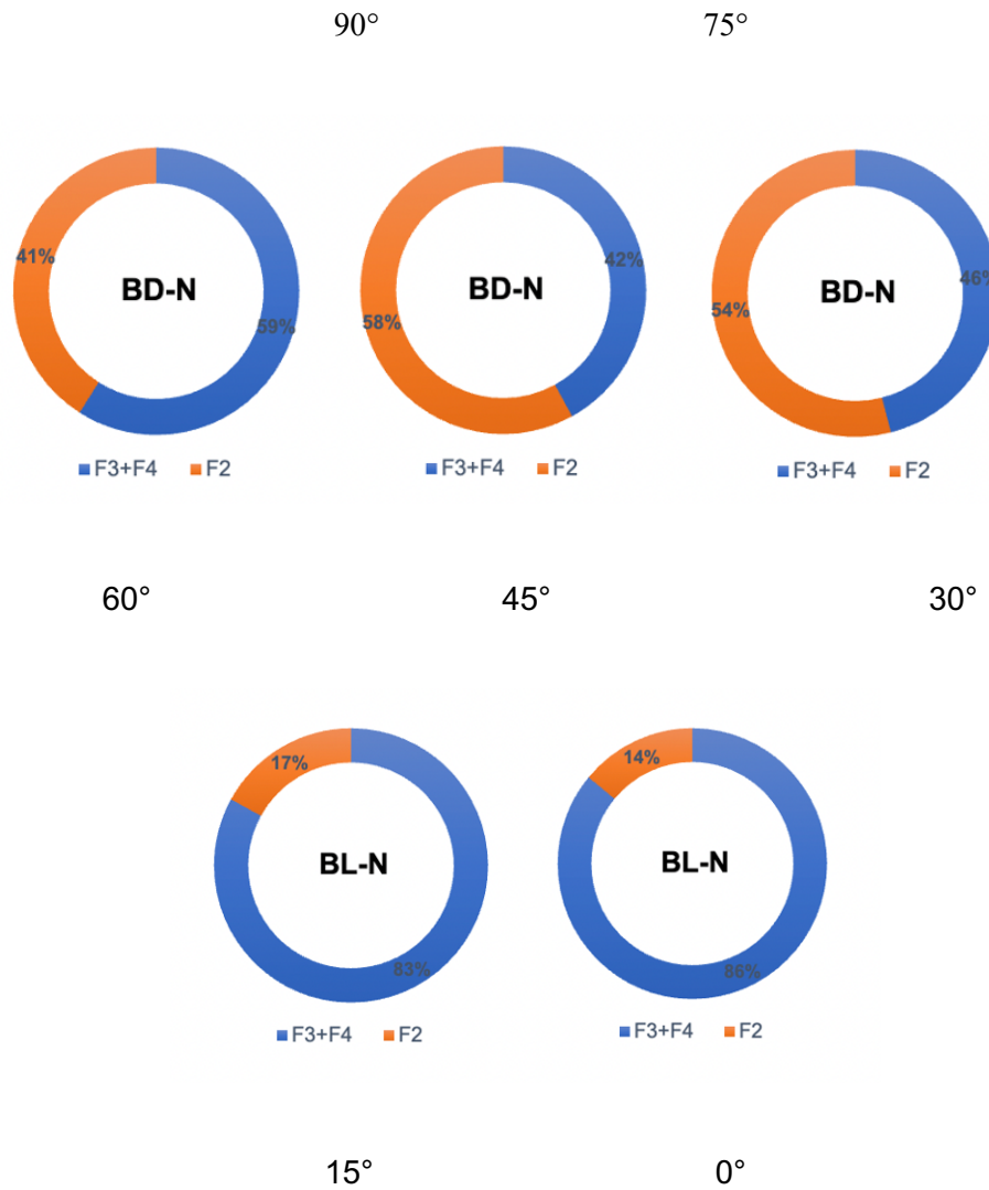
Figure 19 Fracturing modes of the surrounding rock masses with the frequency of varying fracture types under different bedding plane inclinations.
