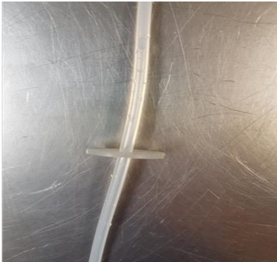
Figure 4. 9: The circular ring that was added to the final chemo patch design for extra outside support
