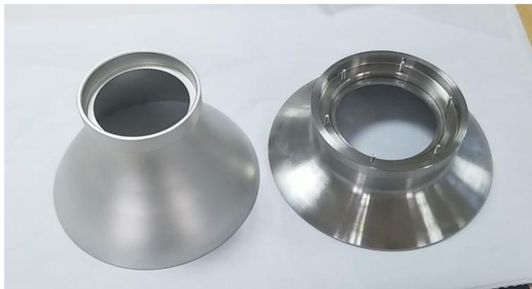
*Figure 5-37. The inlet air duct (left) and outlet air duct (right)*
