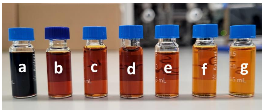
Figure 7.7: Sewage sludge oil samples: (a) raw bio-oil; treated oil over catalysts, (b) TK-341, (c) s -TK-341, (d) hie -Ni/ZSM-5, (e) s - hie -Ni/ZSM-5, (f) Ni/SiO 2 , and (g) s -Ni/SiO 2 treated oil: Oil to catalyst ratio: 10:1, reaction temperature: 350 °C, reaction pressure: 60 bar H 2 , reaction time: 3 hours.
