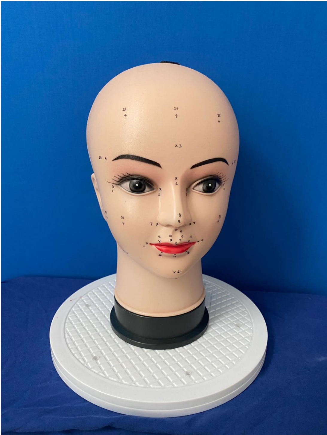
Figure 3.3 Pre-landmarked plastic mannequin head on a turntable, which allowed 360° rotation of the head.
