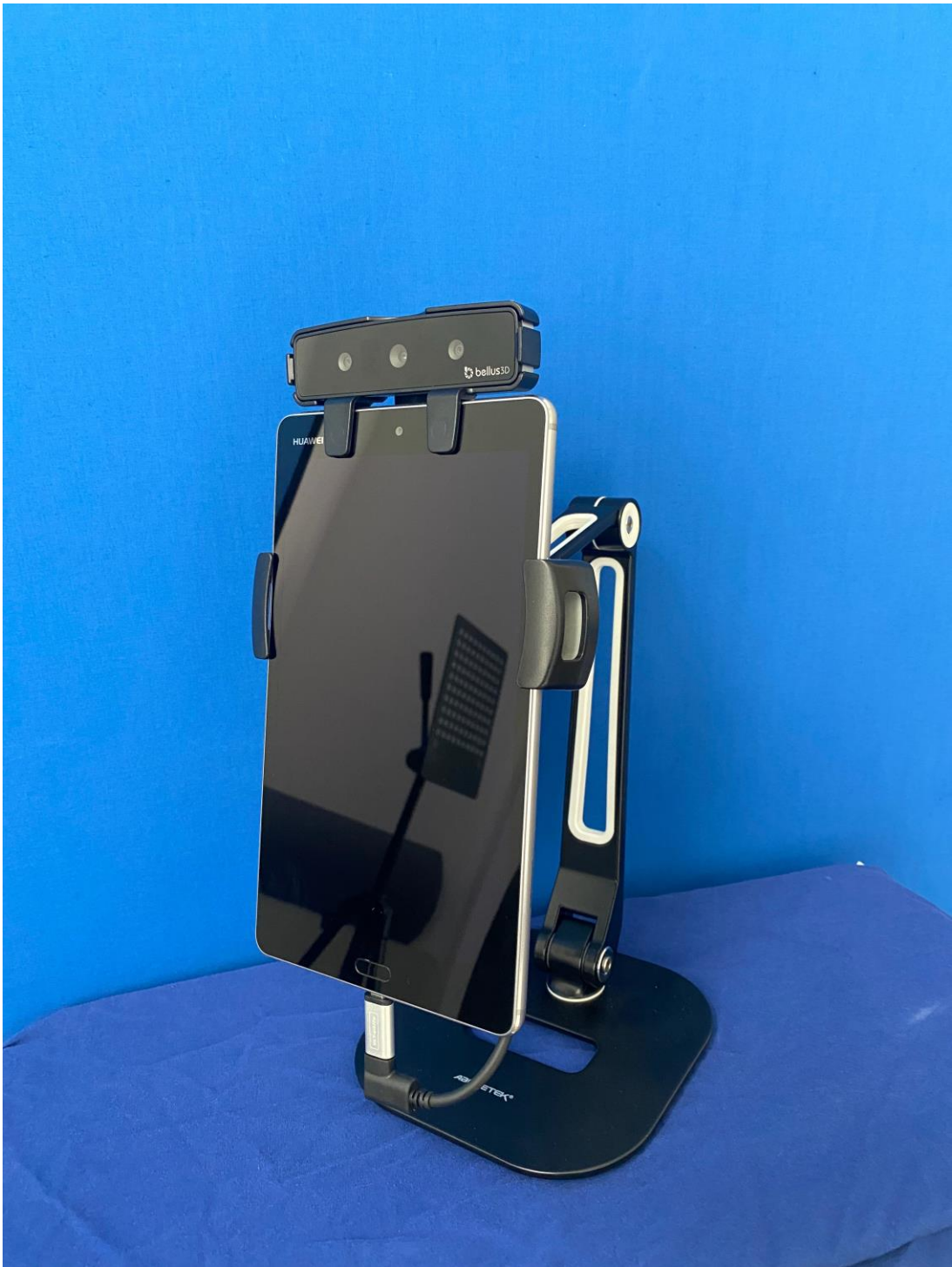
Figure 3.4 Bellus3D system secured to a tablet holder, allowing multi-directional movement of the tablet and camera.
