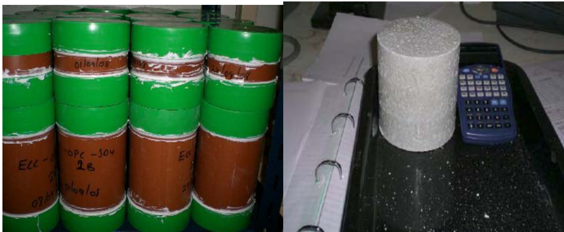
Figure 4:4: Packed, capped and sealed samples in drain pipes, and extruded 100mm sample
