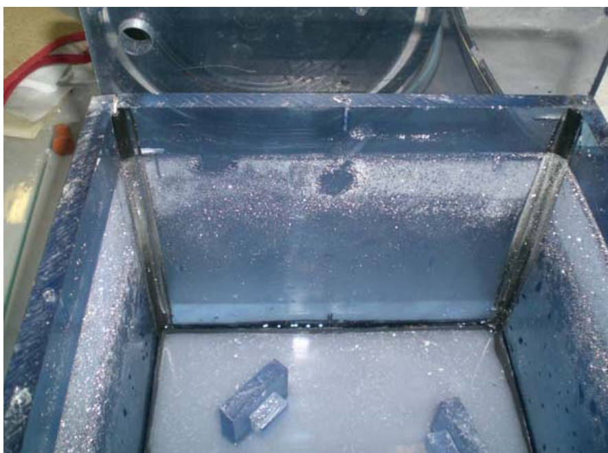
Figure 6:9: Calcium silicate precipitation on walls of monolithic test leaching vessel
