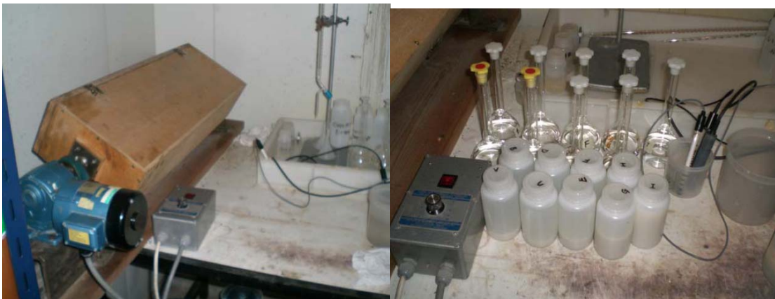
Figure 4.10: Batch extraction end over end shaker, and test fractions during leachant addition
