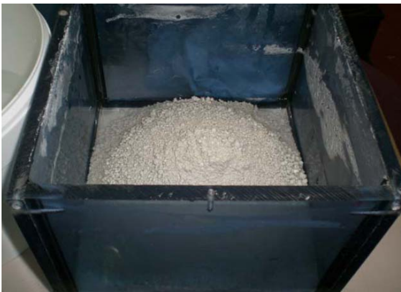
Figure 4.6: Unstabilised clay sample after 6 hours of testing
