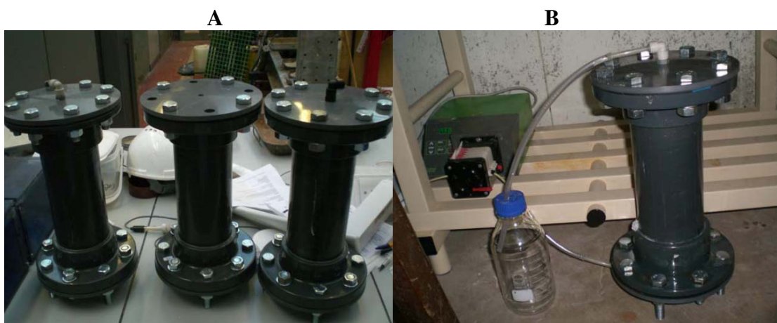
Figure 4.7: Assembled leaching columns, and a complete arrangement of the test apparatus
