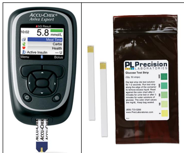
Figure 2.6: An image displaying a blood glucose test (left) and a glucose urine dipstick test (right). Images used from diabetes.co.uk and precision laboratories. [43,44]
