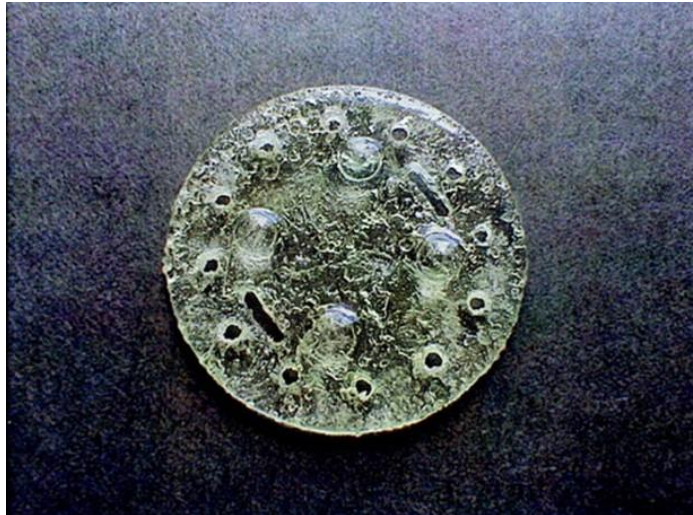
Figure 2.18. fabricated scaffold using stereolithography (SLA). Adopted from M. N. Cooke [125].
