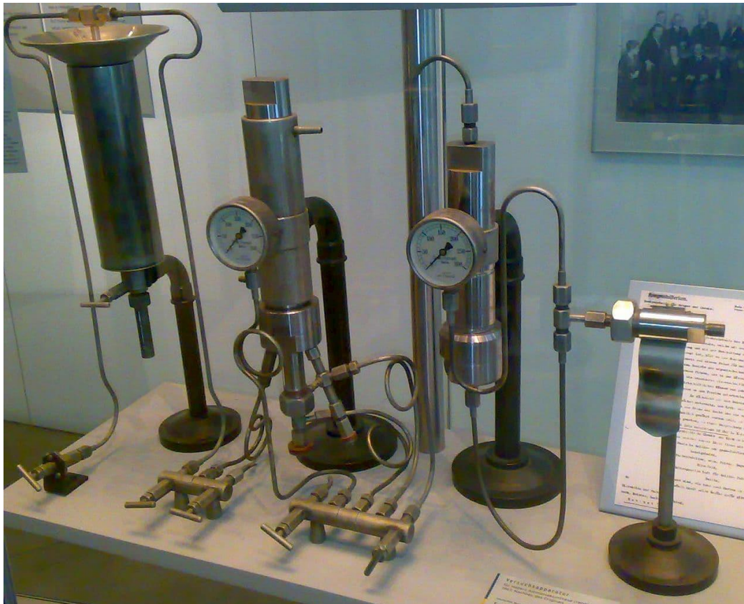
Figure 2: Laboratory reactor used by Fritz Haber to synthesize ammonia ca. 1909.
