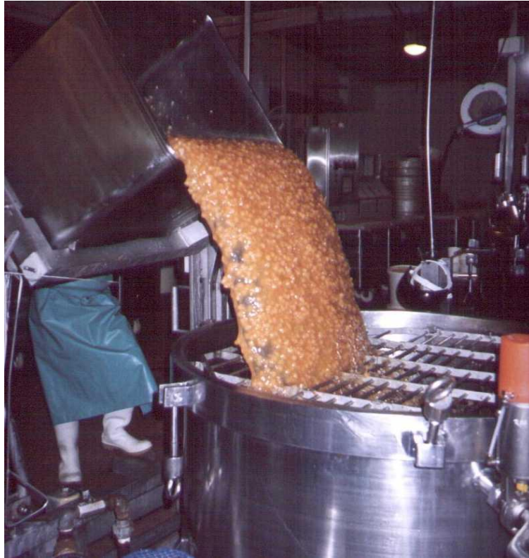
Figure 4.1: 1,000 kg vessel being filled with an apricot product. TTI particles were added after the fruit was in the vessel.
