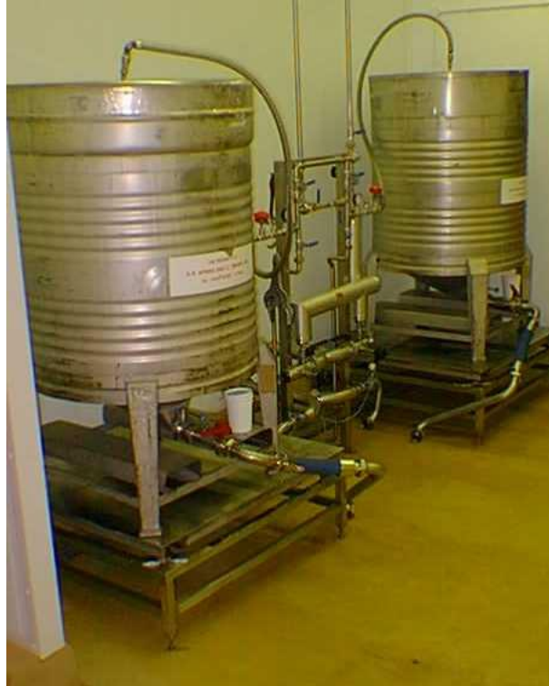
Figure 4.5: Bulk tanks used to store pasteurised fruit preparations. Each of these tanks holds 800 kg of fruit.
