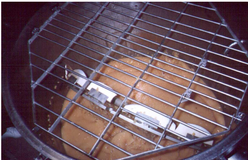
Figure 4.2: Apricot fruit product in the vessel with scraped surface agitator switched on. TTI particles were introduced at this stage by dropping them into the batch.
