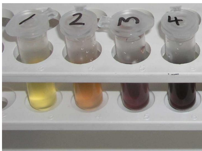
Figure 5.2: Gradation of colour with discontinuous starch/iodine assay. Tube #1 shows a sample with high amylase activity and tube #4 with no activity. Tubes were incubated at 92°C for 15 minutes.
