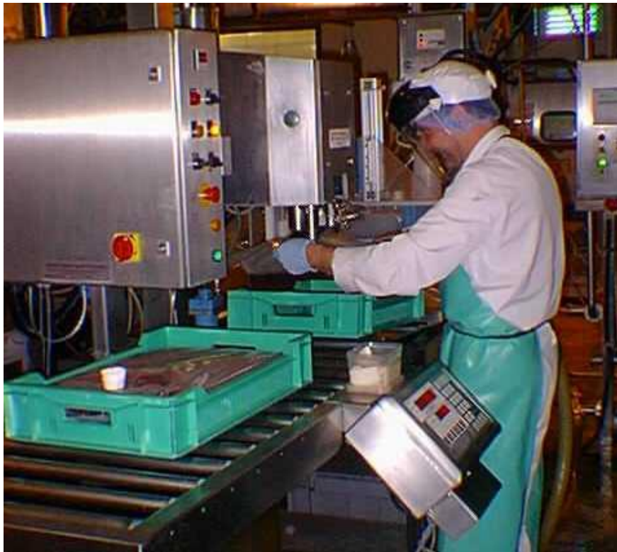
Figure 4.4: Pergal bag filling system showing one filled 8.5 kg bag per tray.
