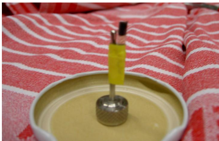
Figure 5.12: Ellab Tracksense logger with a sterilisation TTI tube attached to the measuring tip. (picture courtesy of Masterfoods, Kings Lynn)
