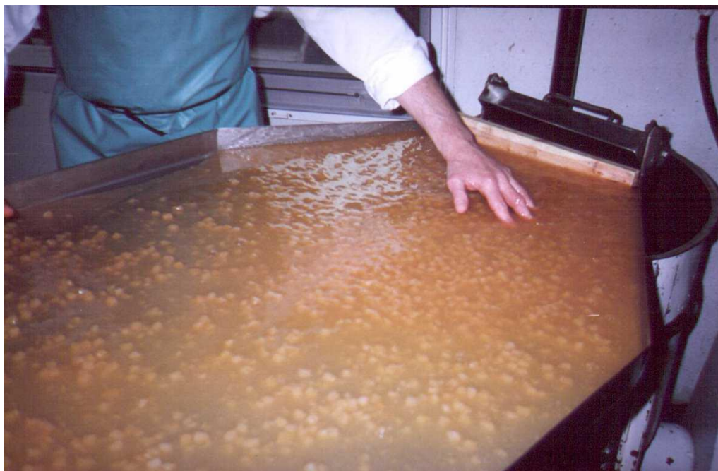
Figure 4.6: Sorting trays used for spreading fruit products into a mono-layer to aid in finding TTI particles. Product shown is an apricot preparation
