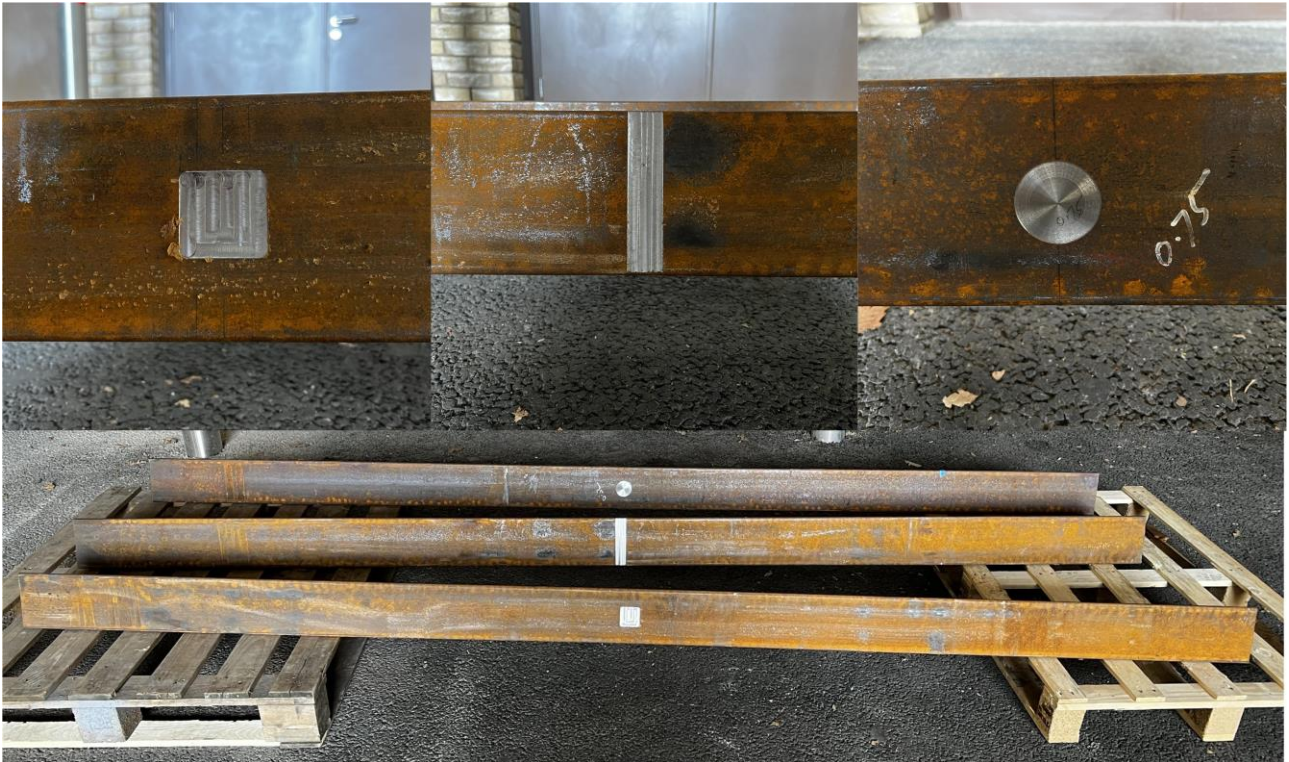
Figure 5.1 Shapes of the rail corrosion
