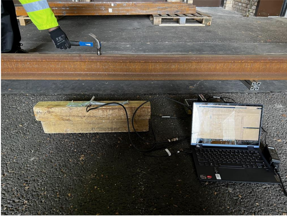
Figure 5.14 Experiment of collecting acoustic signals
