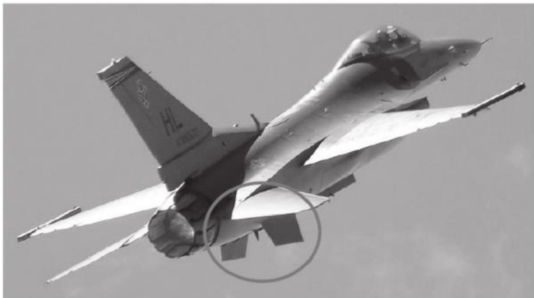
Figure 4.48: Ventral fins of an F-16 Fighting Falcon.
