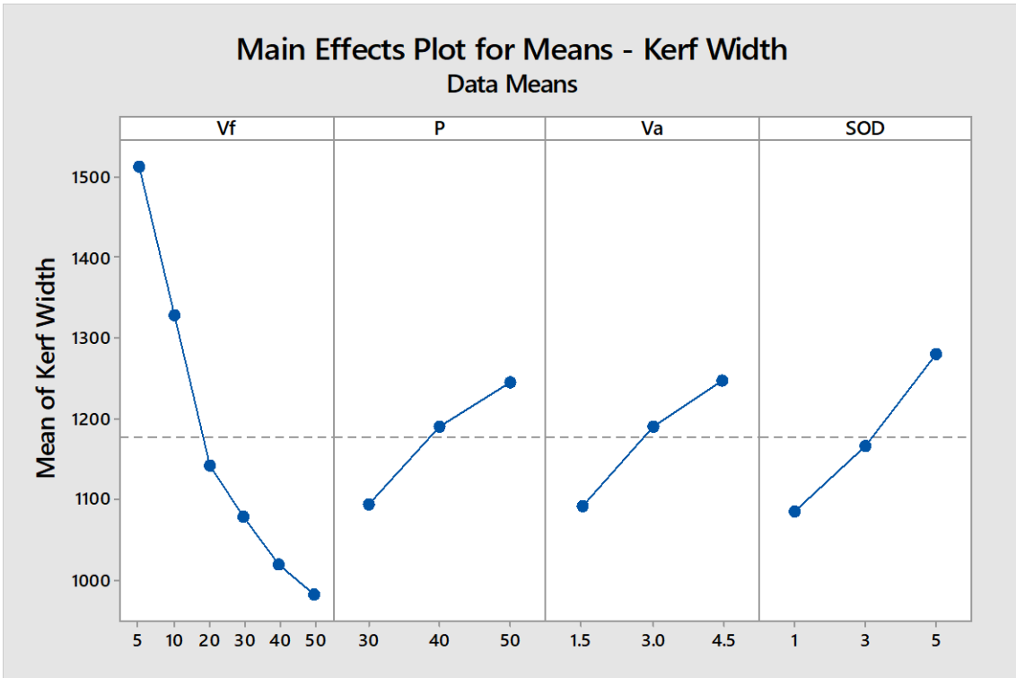
Figure 4.6: Main effect plot of Means for AWJ kerf width.
