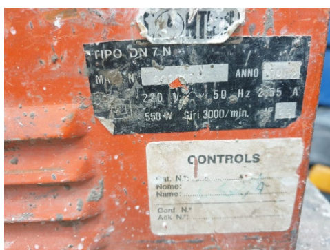
Figure 3-23: Details of Concrete vibrator used during column installation
