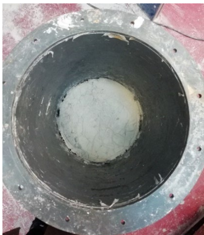
Figure 3-17: Sample after 1 minute of vibratory compaction
