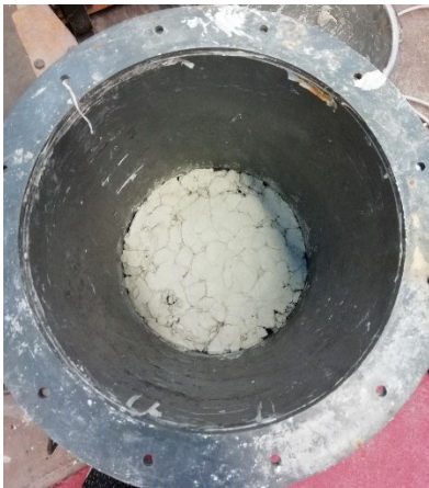
Figure 3-15: Sample after approximately 20 secs of compaction
