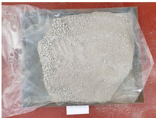
Figure 6-31: APCr after LA testing
