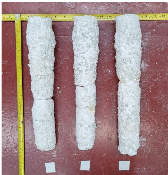
Figure 3-29: Example of Plaster of Paris models of post load column shapes
