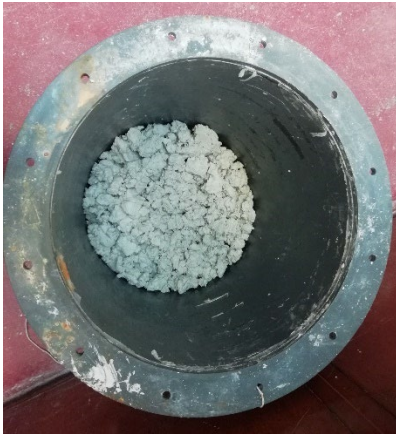
Figure 3-14: Clay prior to compaction using the vibrating hammer
