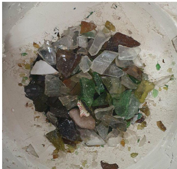
Figure 6-23: Images of the columns post load. Wet material can be seen in the images of the granite (top) and APCr (centre) whilst the container glass appears dry (bottom).
