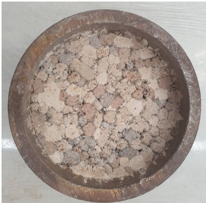
Figure 6-30: APCr after aggregate impact (AIV) test
