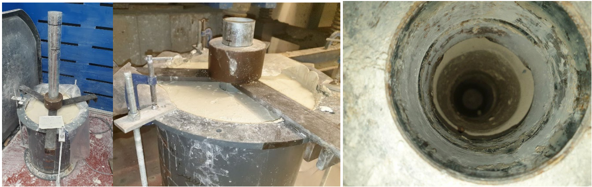
Figure 3-20: From left to right: (a) Centralising frame and installation tube, (b) imaging showing how centralising frame is fixed to container, (c) Empty bore
