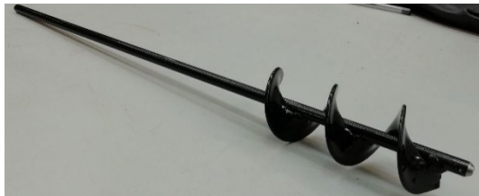
Figure 3-22: Auger used to remove clay from inside tube
