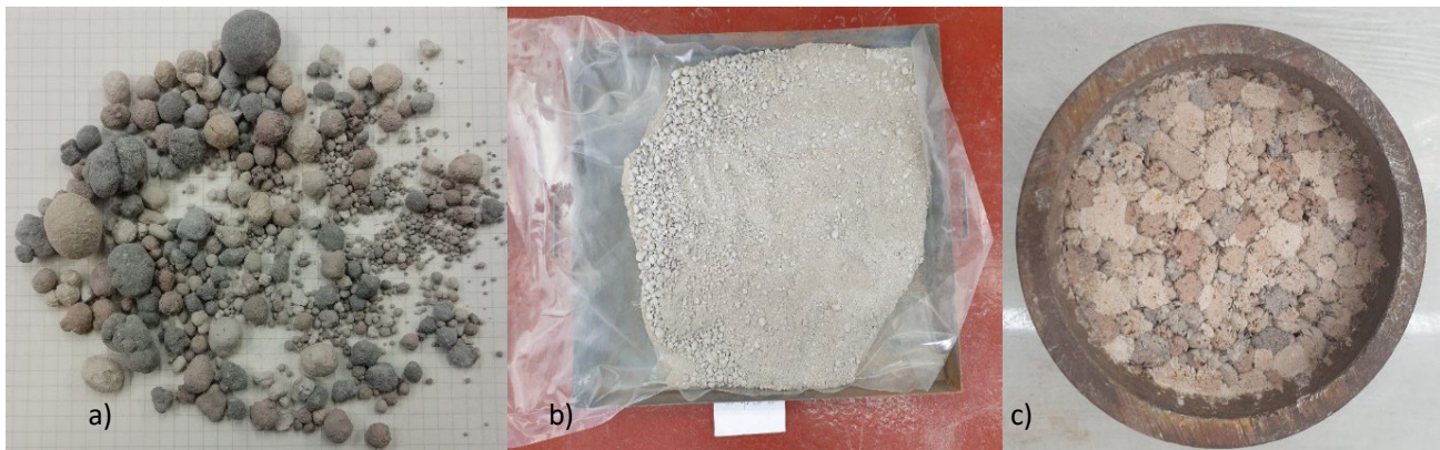
Figure 4-26: Change in APCr with testing: (a) Sample of APCr before testing (previously used in Figure 5-4) (b) sample of APCr after LA testing (reproduced in Figure 6.37) and (c) sample of APCr after AIV testing (reproduced in Figure 6.33)
