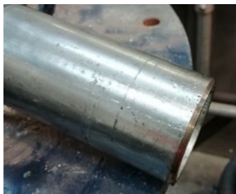
Figure 3-21: Chamfered edge of installation tube
