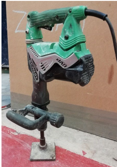
Figure 3-13: 900 w Vibro-compaction hammer
