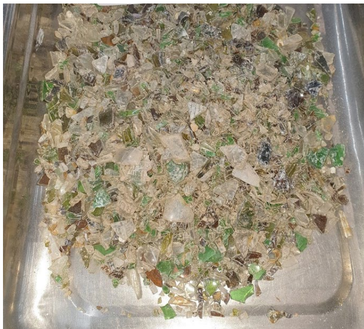
Figure 6-22: Clay smeared container glass aggregate after load test
