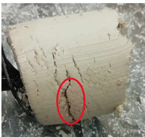
Figure 3-12: Visible layers within soil structure
