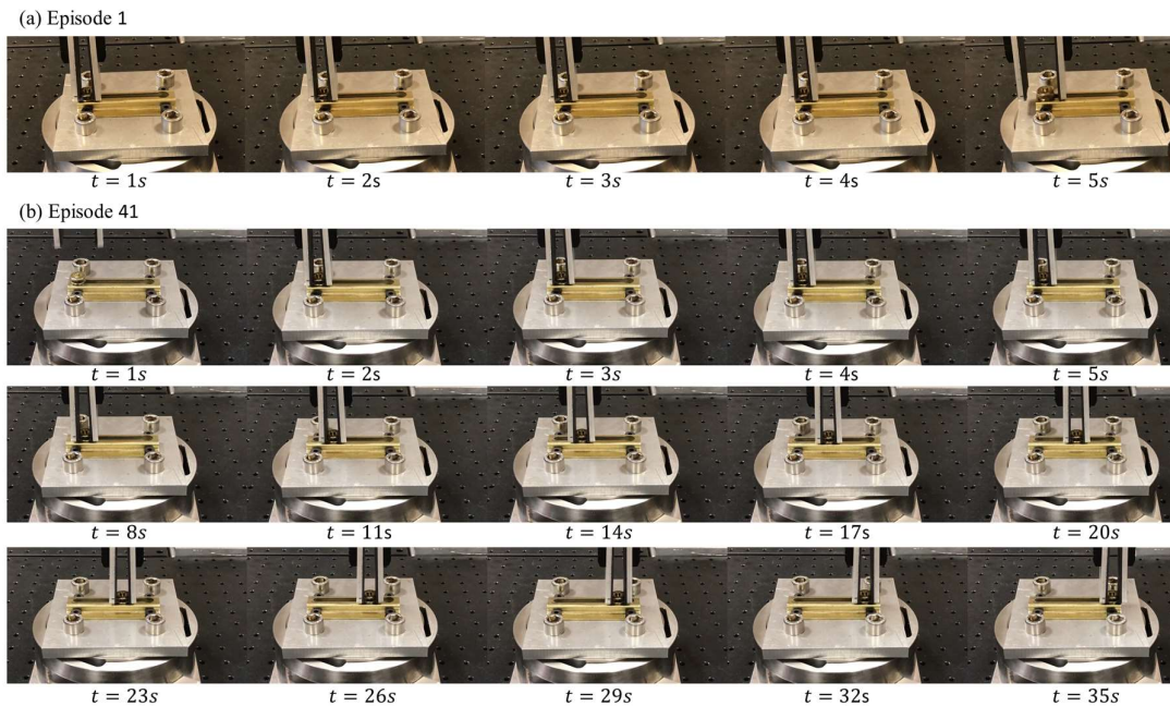
Figure 3.3: Photographs taken from the footage of one training session: (a) at the beginning of the episode, (b) after several episodes of training. It can be seen that the robot learned the sliding task by trial and error. (Note: t in here represents the real time of the video, not the time step in MDP.)
