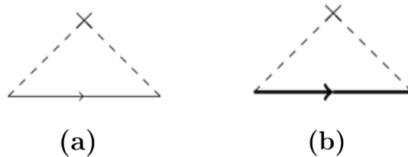
Figure 3.7: The self-energy in the presence of disorder. The thin (thick) solid line represents the free (full) electronic Green’s function and the dashed line represents the impurity potential, U . The cross represents that the scattering occurs from the same atom in this model. (a) : The first order term in the self-energy. (b) : The full self-energy.
