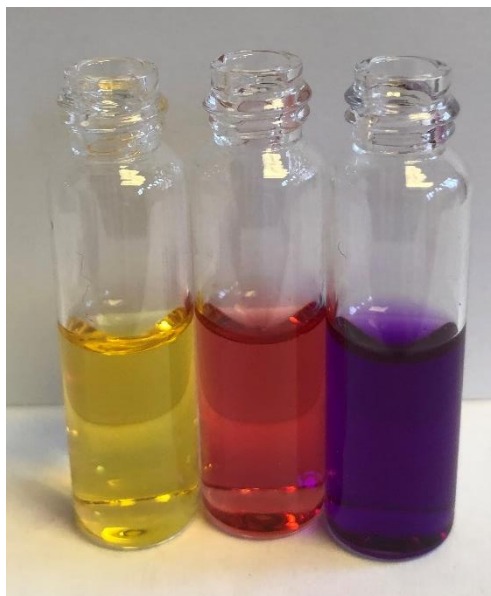
Figure 4.4 – Alizarin Red S ( 2.5 \times 10^{-4} \text{ mol dm}^{-3} ) in sodium phosphate buffer at pH 4.0, 7.4 and 12.0 (left to right).
