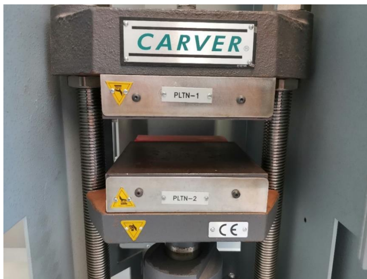
Figure 3-4: Hot press machine for multiple tape lamination.
