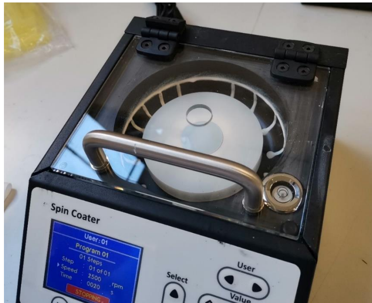
Figure 3-5: Vacuum-free spin coater used for thin GDC film fabrication.
