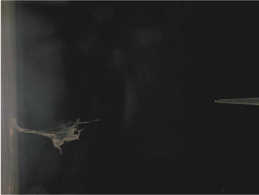
Figure 122. Mesh becomes larger with subsequent deposition of fibres.
