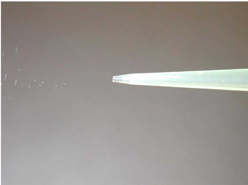
d. Drop is ejected and electrospinning jet forms immediately and continues the process.
