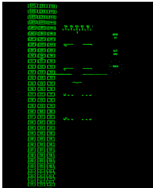
Figure 42. Co-ordinated numbered boxes were placed in the same position of each optic. When the HMD was well aligned, some inherent distortion was apparent, as indicated by the diplopic boxes.
